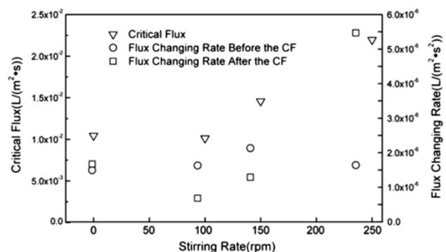
Fig. 2. The influence of stirring rate on critical flux and the membrane fouling for activated sludge (MLSS concentration of 4,500 mg/L and temperature of 21°C).
