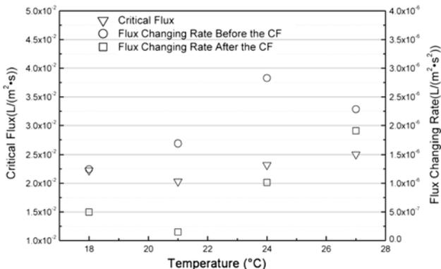
Fig. 3. The influence of temperature on critical flux and the membrane fouling for activated sludge (MLSS concentration of 4,500 mg/L and stirring rate of 200 rpm).
