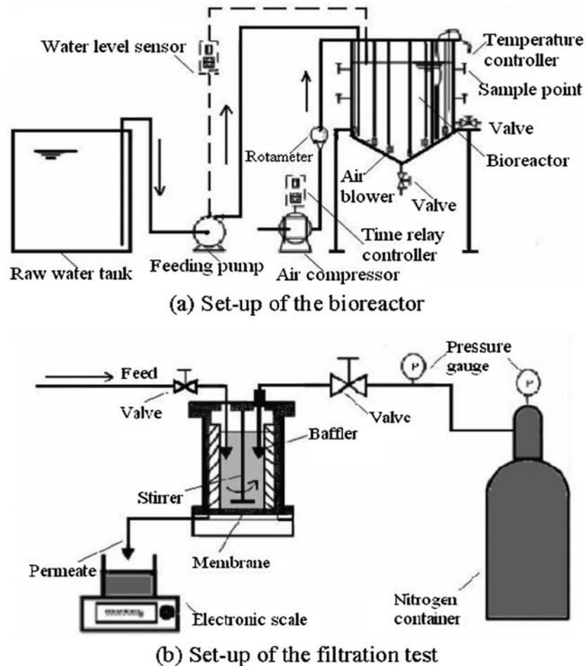
Fig. 1. Schematic diagram of the experimental system.
