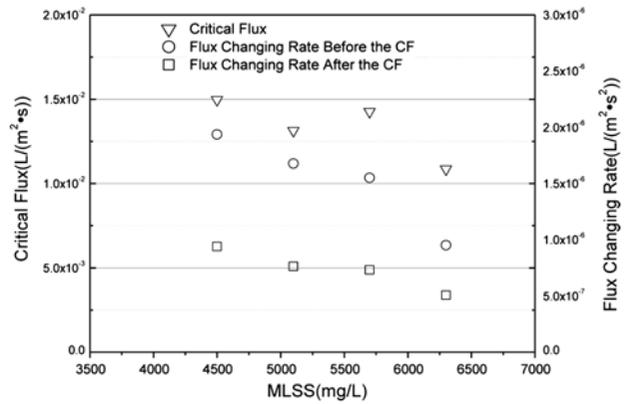
Fig. 4. The influence of the concentration of MLSS on critical flux and the membrane fouling for activated sludge (temperature of 21°C and stirring rate of 200 rpm).
