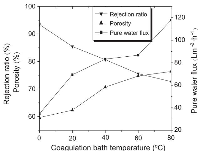
Fig. 4. Effect of coagulation bath temperature on membrane's pure water flux, BSA retention and porosity.
