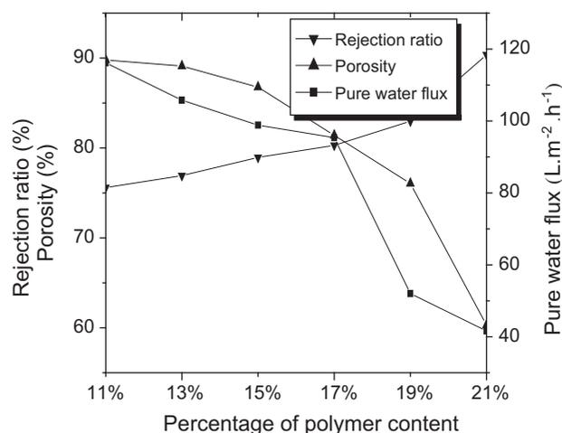
Fig. 2. Effect of percentage of polymer content on membrane's pure water flux, BSA retention and porosity.
