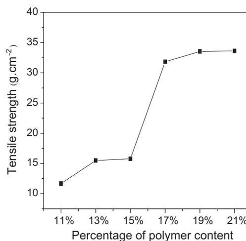
Fig. 3. Effect of percentage of polymer content on membrane's tensile strength.
