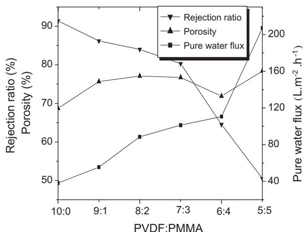
Fig. 1. Effect of PVDF/PMMA blending ratio on membrane's pure water flux, BSA retention and porosity.
