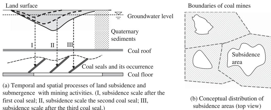
Fig. 1. Occurrence processes of land subsidence and submergence.
