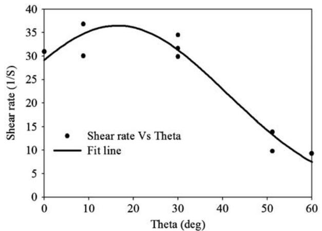
Fig. 8. Result of response surface, showing the relationship between angle of guided baffle and shear rate at the bottom of the sedimentation tank.
