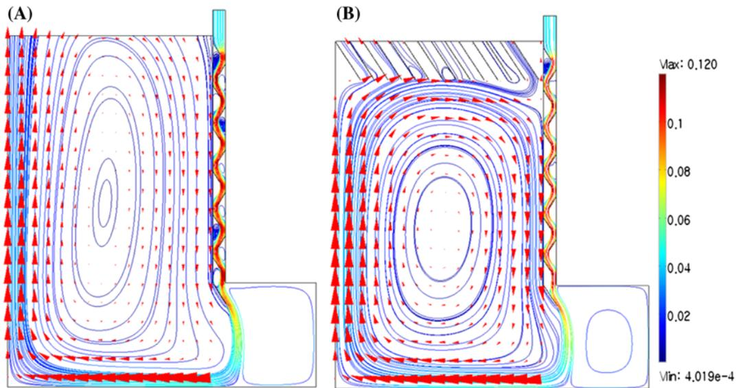
Fig. 6. Effect of inclined panel on stability of rising flow without inclined panel (A) and with inclined chamber (B).
