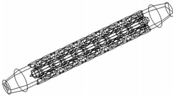
Fig. 2. Geometric view of the inline static mixer.
