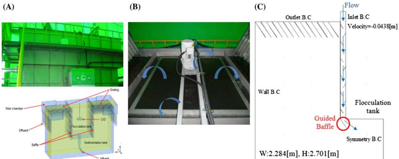
Fig. 3. Schematic of sedimentation: (A) front view (B) top view, and (C) cross section (W: width, H: height).
