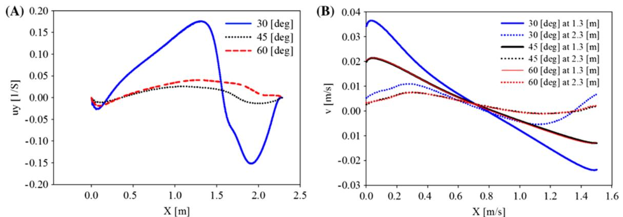
Fig. 9. Comparisons between the sedimentation performance among different angles of guided baffle (30°, 45°, and 60°), (A) shear rate (B) rising velocity.
