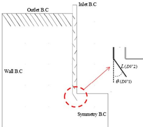
Fig. 7. DV, DV1: angle of guided baffle, DV2: length of guided baffle.
