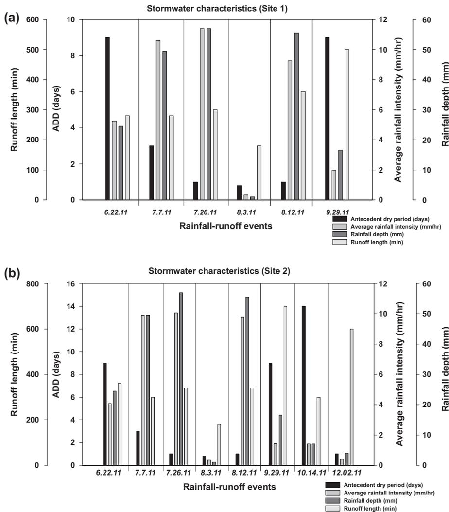
Fig. 2. Rainfall-runoff characteristics.
