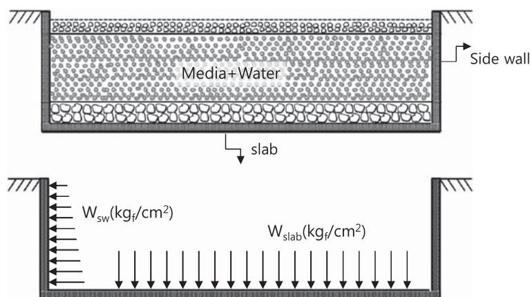
Fig. 5. The schematic diagram of the load from filter media layer.
