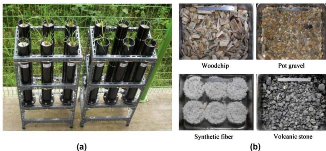
Fig. 1. Photos of the VF stormwater wetlands and the media used in this study.
