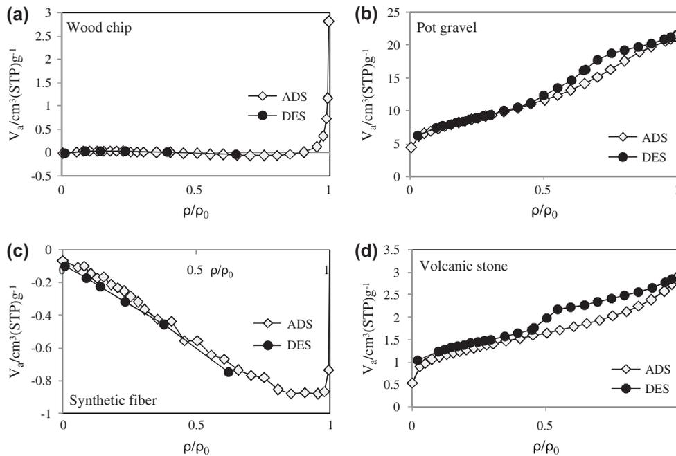
Fig. 3. Adsorption/desorption isotherms of four types of media.
