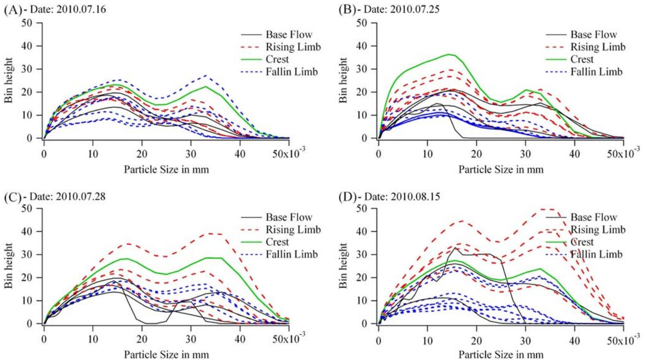
Fig. 4. Bin height of each particle size in accordance with hydrograph. Vertical axis indicates the bin height and horizontal axis indicates the particle size in mm.
