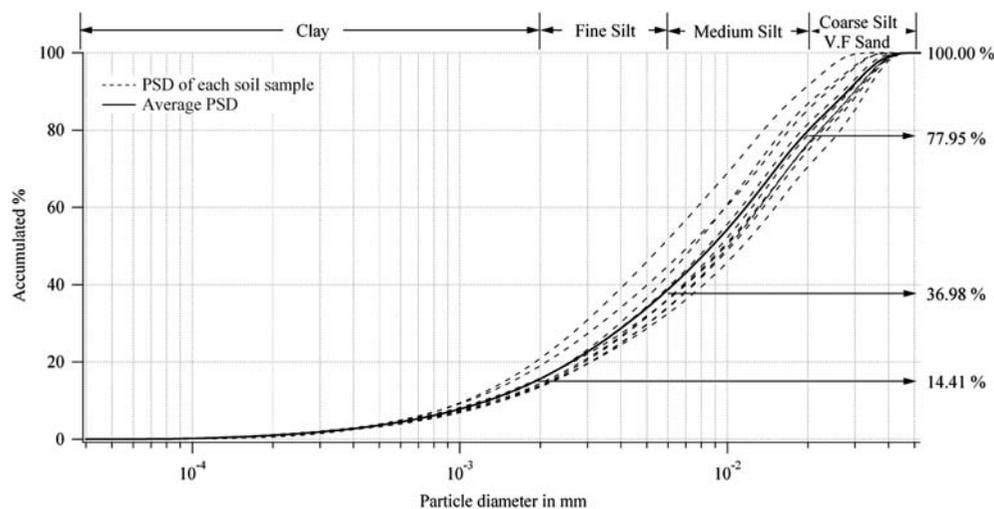
Fig. 2. PSD curves for soil samples collected from drainage area. In the graph, the vertical axis indicates the particle diameter in mm and vertical axis indicates the accumulated volume.
