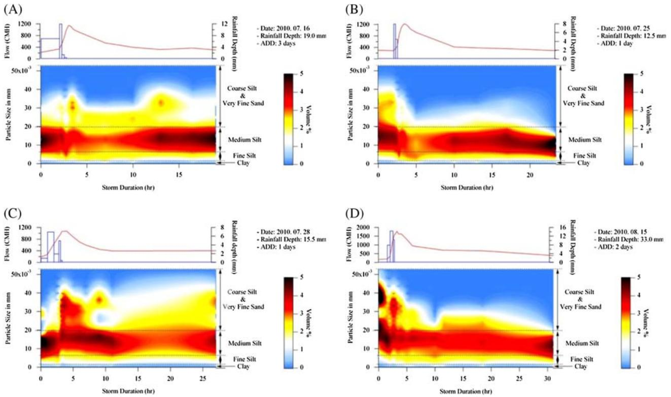
Fig. 3. Volume percentage of each particle size for four field experiments. Top panel indicates the flow and the rainfall depth and bottom panel indicates the contour plot for particle volume percentages with respect to storm duration.
