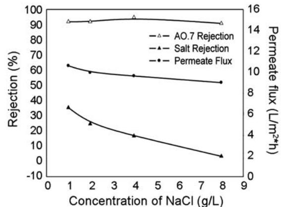
Fig. 2. Rejection and flux of Acid orange 7/NaCl mixture vs. the concentration of NaCl.
