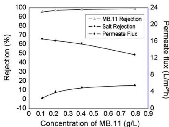
Fig. 6. Rejection and flux of Mordant Black 11/NaCl mixture vs. the concentration of dye.
