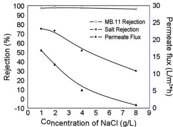
Fig. 3. Rejection and flux of Mordant Black 11/NaCl mixture vs. the concentration of NaCl.
