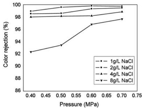
Fig. 9. Color removal of Mordant black 11/NaCl mixture vs. pressure.
