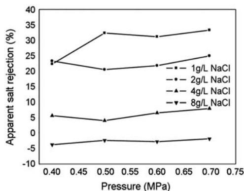
Fig. 8. Apparent salt rejection of Mordant black 11/NaCl mixture vs. pressure.
