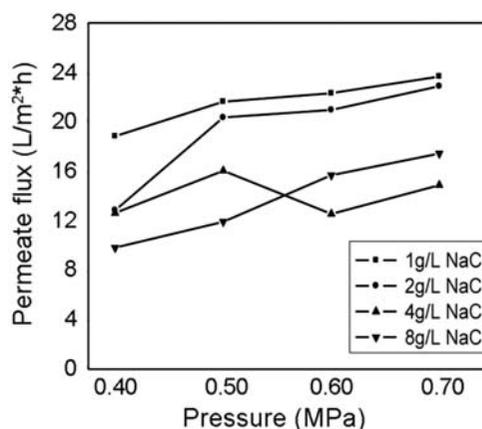
Fig. 7. Permeate flux of Mordant black 11/NaCl mixture vs. pressure.
