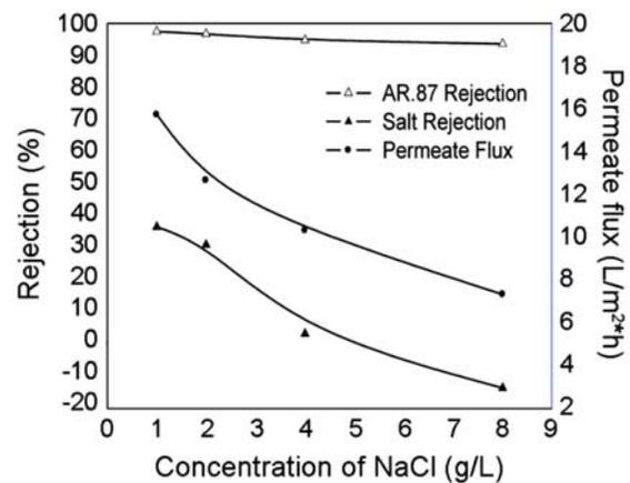
Fig. 1. Rejection and flux of Acid red 87/NaCl mixture vs. the concentration of NaCl.
