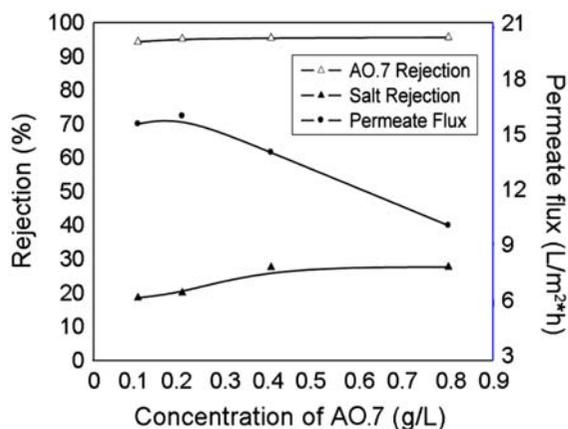
Fig. 5. Rejection and flux of Acid orange 7/NaCl mixture vs. the concentration of dye.
