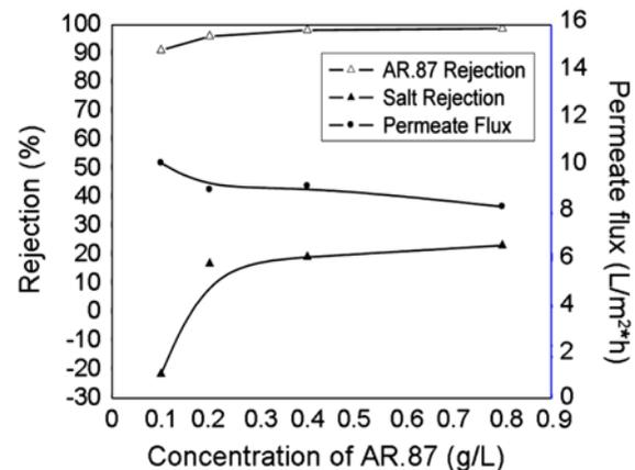
Fig. 4. Rejection and flux of Acid red 87/NaCl mixture vs. the concentration of dye.
