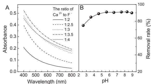
Fig. 1. A—the optimum dosages of  $\text{F}^-$  addition in the process of becoming  $\text{CaF}_2$  in the presence of 0.040 mol/L  $\text{Ca}^{2+}$ ; B—Effect of pH on assembly aggregation of CFA. (0.120 mol/L  $\text{F}^-$ , 0.040 mol/L  $\text{Ca}^{2+}$ , 1.5 mmol/L AR138).
