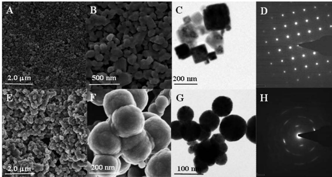
Fig. 2. SEM images of CaF<sub>2</sub>-only (A, B) and CFA hybrid particles (E, F), HRTEM of CaF<sub>2</sub>-only (C), CFA hybrid particles (G) and EDX images of CaF<sub>2</sub>-only (D) and CFA hybrid particles (H).
