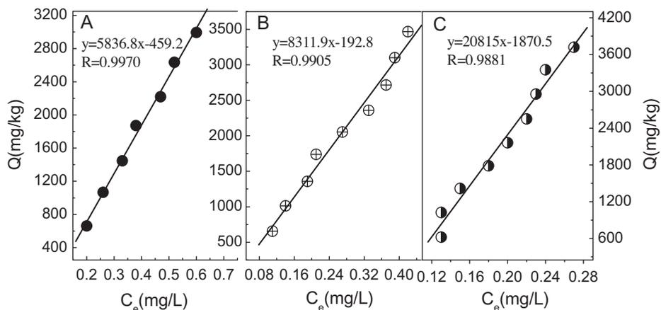
Fig. 4. Adsorptions of PCB029 (A), PCB101 (B), and PCB180 (C) 0.06% CFA was added.
