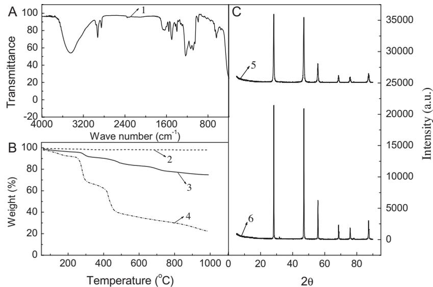
Fig. 3. A-IR spectra of CFA (curve 1), B-different particles TGA for CaF<sub>2</sub>-only (curve 2), CFA (curve 3) and AR138-only (curve 4) and C-XRD of CaF<sub>2</sub>-only (curve 5) and CFA (curve 6).
