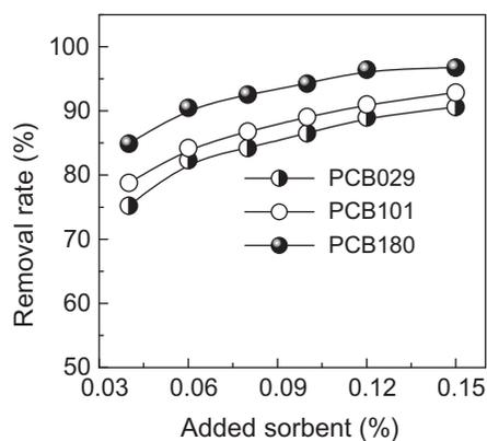
Fig. 7. The removal rate of PCBs in the polluted water treated with CFA sorbent.
