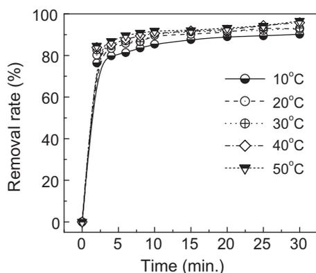
Fig. 6. Effect of temperature and time on the removal rate of PCB101 absorbed by 0.05% CFA hybrid particles.
