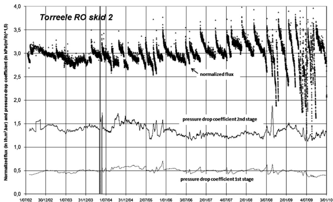
Fig. 3. Normalized performance of RO skid 2 from start-up until 31 March 2010.
