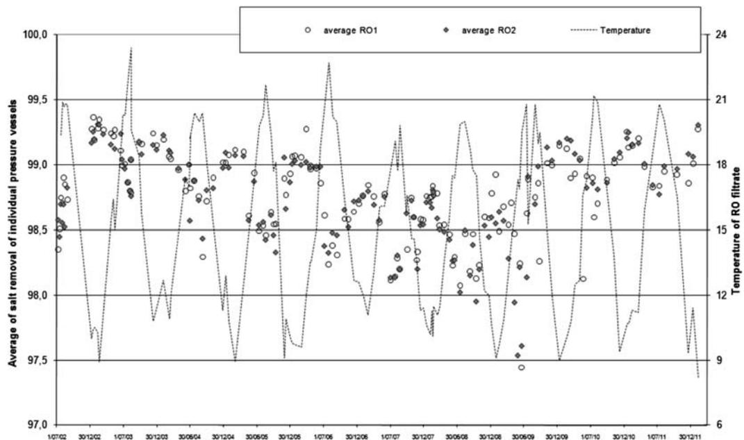
Fig. 2. Salt removal (average of results of every RO pressure vessel and based on conductivity) from start-up until March 2012.
