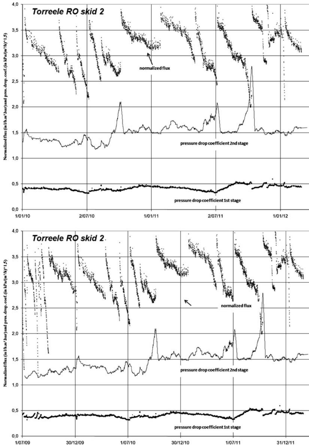
Fig. 4. Normalized performance of RO skid 2 from start-up from mid-2009 until March, 2012.
