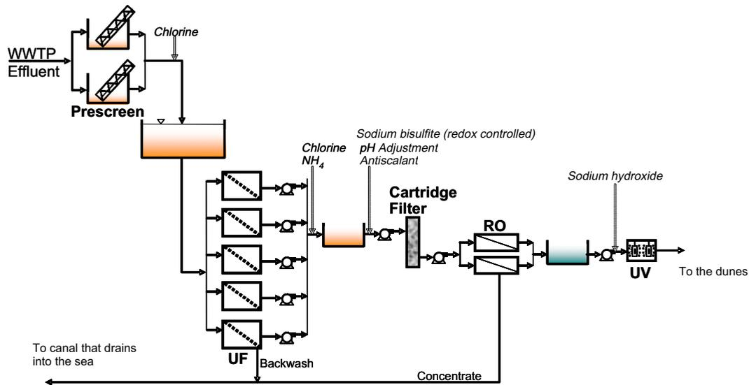
Fig. 1. Process scheme of the Torreele plant.
