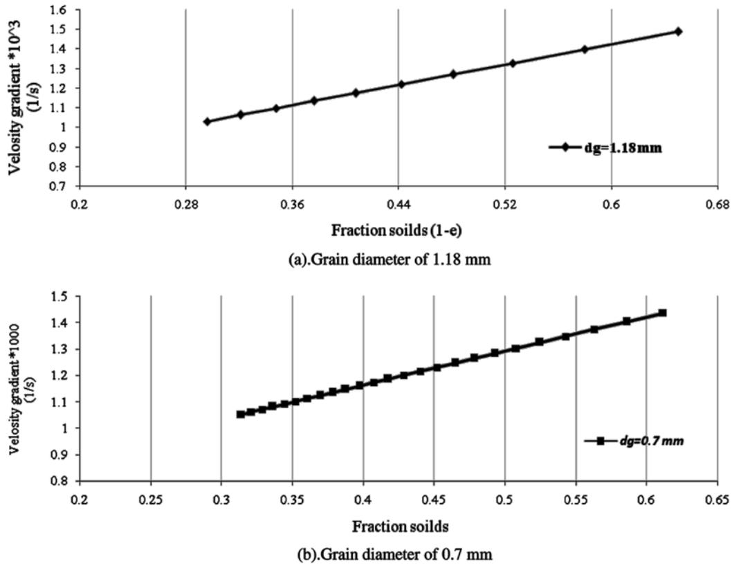
Fig. 5. Effect of velocity gradient on media grain size. (a) Grain diameter of 1.18 mm and (b) Grain diameter of 0.7 mm.
