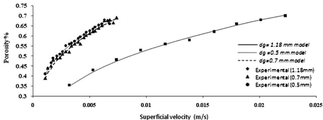
Fig. 3. Predicated and measured porosity vs. superficial velocity for different grains sand.
