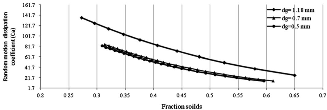
Fig. 7. Random motion dissipation coefficient vs. fraction solids.
