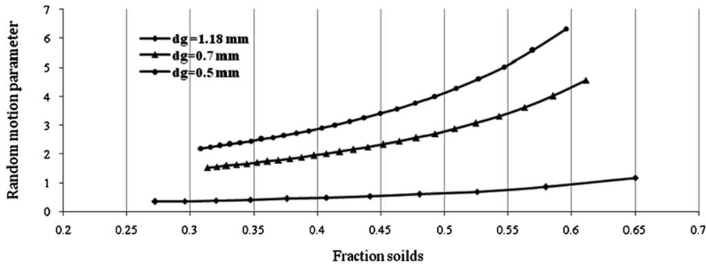
Fig. 8. Random motion parameter vs. fraction solids.
