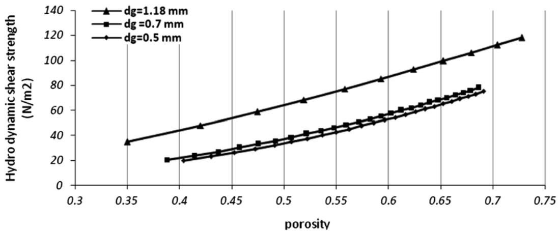
Fig. 6. Fluid shear strength vs. porosity.
