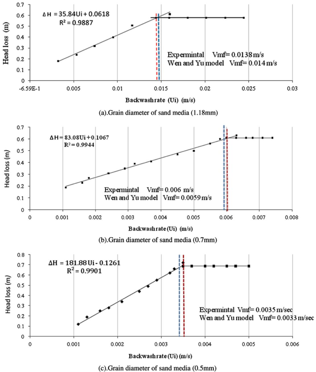
Fig. 4. Minimum fluidization velocity for different grain size. (a) Grain diameter of sand media (1.18 mm); (b) Grain diameter of sand media (0.7 mm); and (c) Grain diameter of sand media (0.5 mm).
