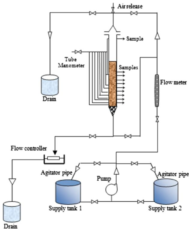
Fig. 1. Schematic diagram of deep bed water filter with all main parts.
