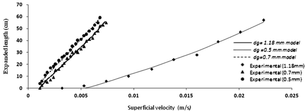
Fig. 2. Predicated and measured expanded bed length vs. superficial velocity for different grains sand.
