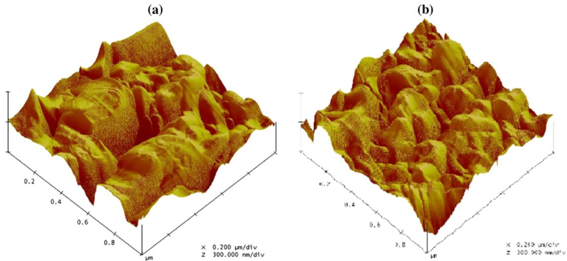
Fig. 3. AFM micrographs of the membrane surface of (a) polyamide AMC and (b) polyamide polysulfone membrane.
