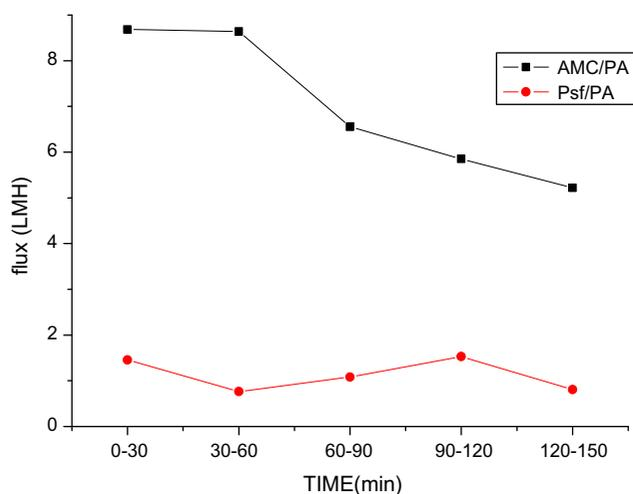
Fig. 4. Graph of FO performance of AMC and polysulfone for 150 min.
