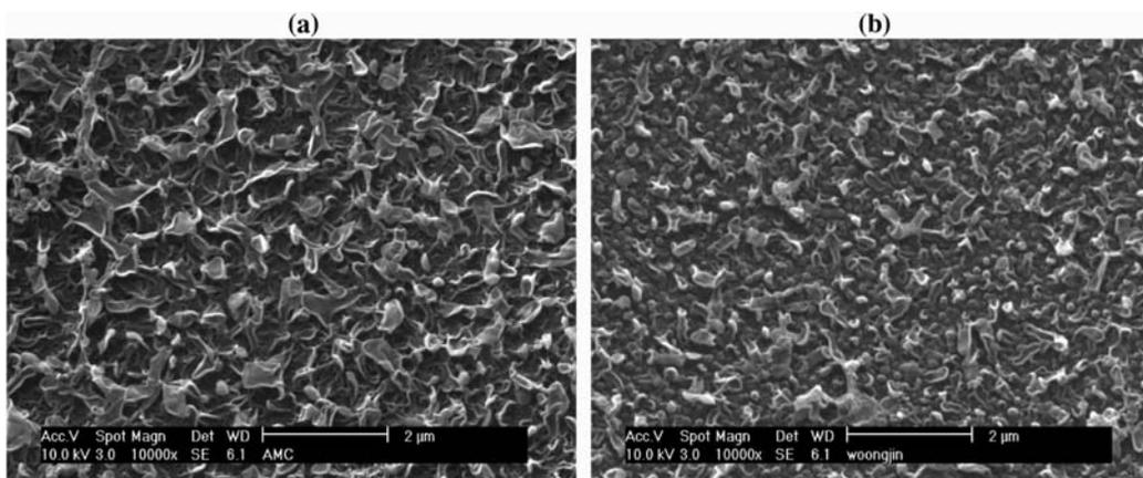
Fig. 2. SEM micrographs of the membrane surface of (a) polyamide AMC and (b) polyamide polysulfone membrane.
