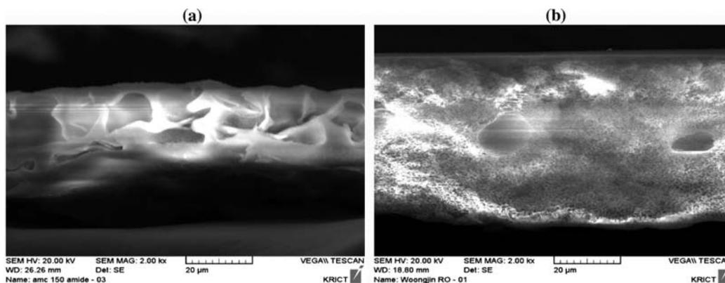
Fig. 1. Cross-sectional SEM images of (a) polyamide AMC and (b) polyamide polysulfone membrane.
