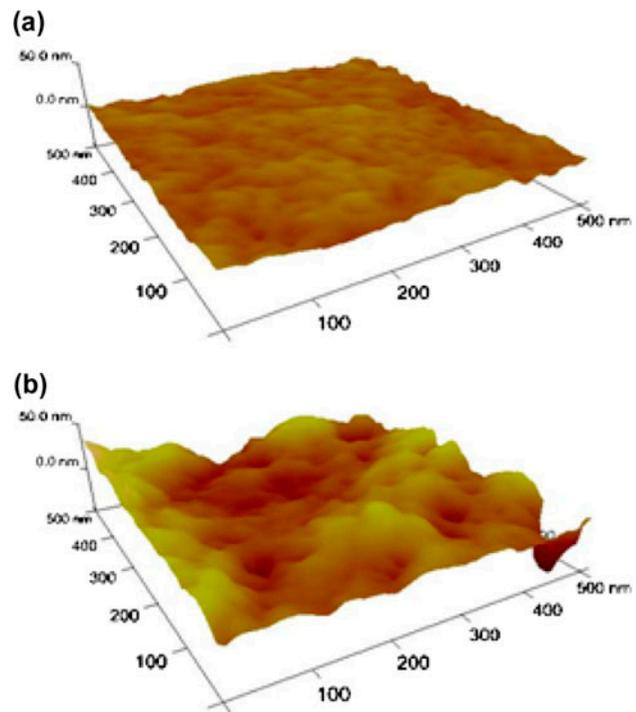
Fig. 10. AFM images of (a) AMC and (b) PVDF membrane.
