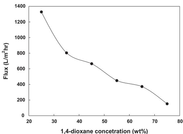
Fig. 7. Effect of 1,4-dioxane on water flux.
