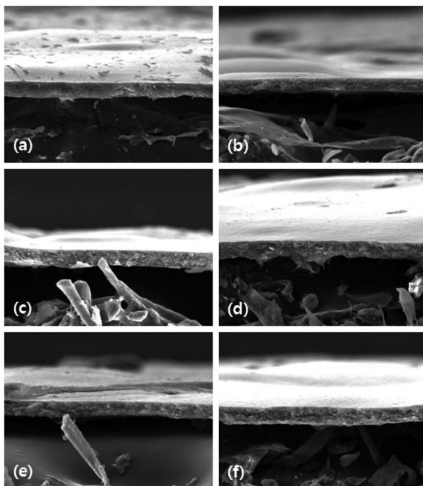
Fig. 8. Effect of 1,4-dioxane and acetone concentration on morphology of AMC membranes (1,4-dioxane/acetone); (a) 1:4 (b) 1:3 (c) 1:2 (d) 1:1 (e) 2:1 (f) 3:1.
