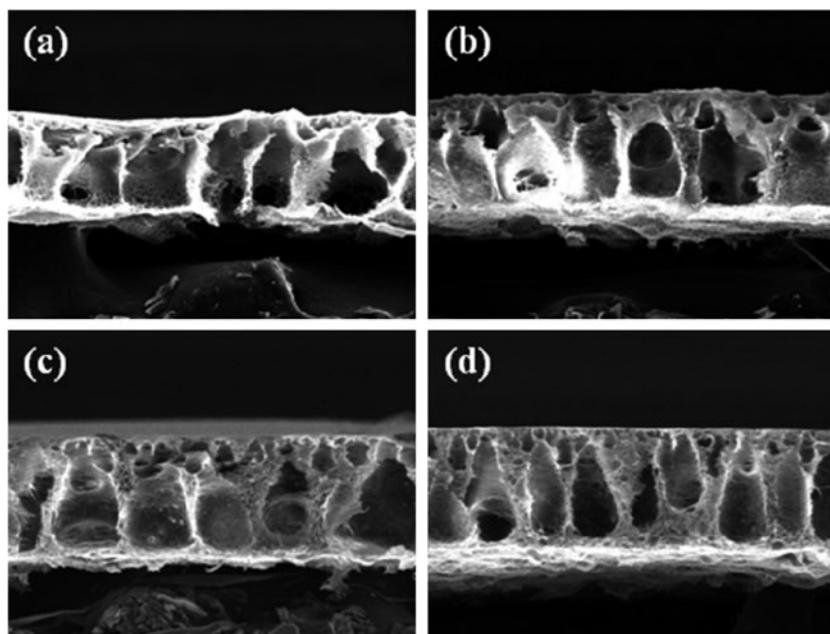
Fig. 4. Effect of AMC concentration on morphology of the synthesized flat sheet membrane; (a) AMC 7 wt% (b) AMC 10 wt% (c) AMC 12 wt% (d) AMC 14 wt%.
