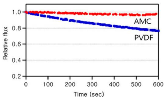
Fig. 9. Protein fouling of the AMC membrane.
