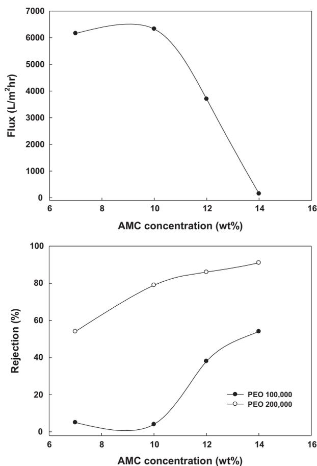
Fig. 5. Effect of AMC concentration on water flux and rejection.
