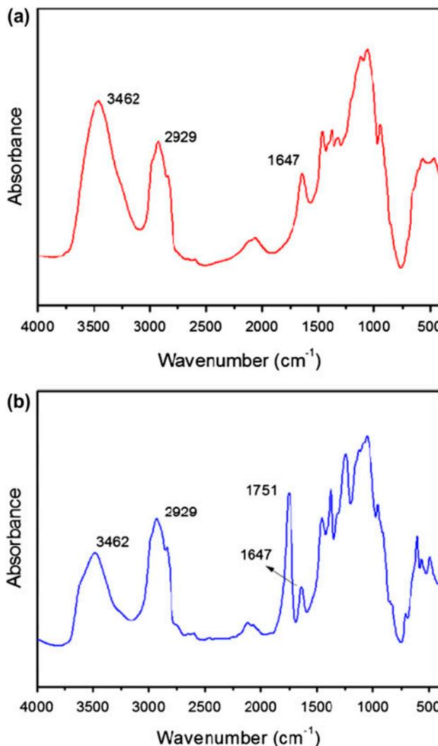
Fig. 3. FT-IR spectra of (a) methyl cellulose and (b) AMC.
