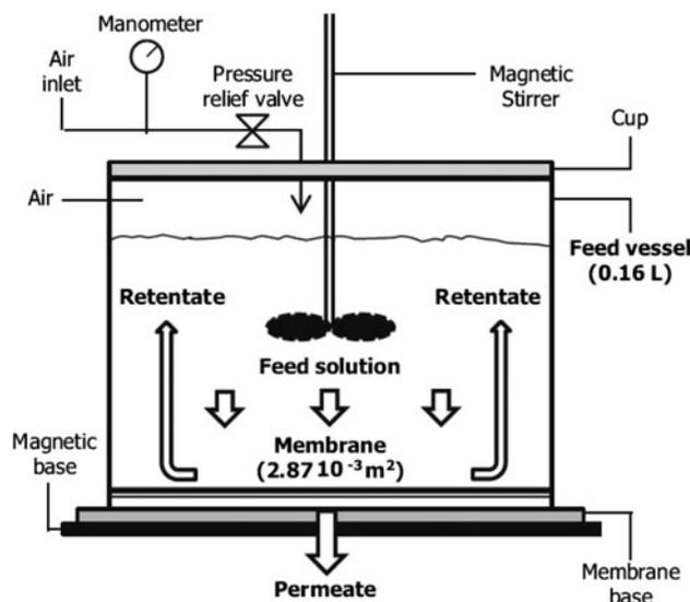
Fig. 2. Schematic diagram of the experimental UF unit.
