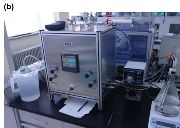
Fig. 2. Laboratory-scale FO system (a) schematic diagram and (b) photograph of the system.
