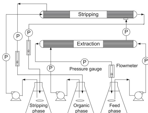
Fig. 1. Schematic representation of experimental setup for extraction and re-extraction in hollow fiber contactors.
