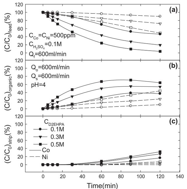
Fig. 4. Time profiles of the extraction and re-extraction for Co(II) and Ni(II) in HFMCs at different  $\text{D}_2\text{EHPA}$  concentrations: (a) feed phase, (b) organic phase, and (c) strip phase.
