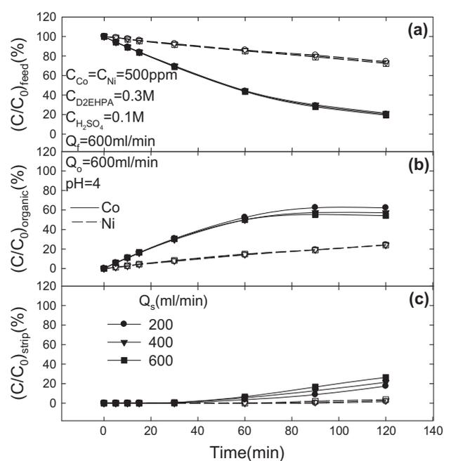
Fig. 8. Time profiles of extraction and re-extraction for Co(II) and Ni(II) in HFMCs at different flow rates of strip phase: (a) feed phase, (b) organic phase, and (c) strip phase.
