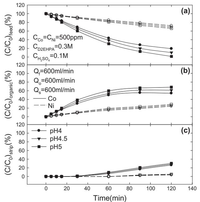
Fig. 3. Time profiles of the extraction and re-extraction for Co(II) and Ni(II) with  $\text{D}_2\text{EHPA}$  in HFMCs at different feed pH: (a) feed phase, (b) organic phase, and (c) strip phase.
