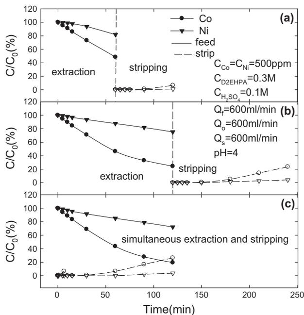
Fig. 9. Time profiles of the extraction and re-extraction for Co(II) and Ni(II) in HFMCs (a) using two-stage (2 h operation), (b) using two-stage (4-h operation), and (c) one-stage (2-h operation).
