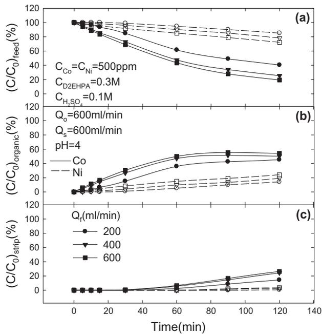
Fig. 6. Time profiles of extraction and re-extraction of Co(II) and Ni(II) in HFMCs at different flow rates of feed phase: (a) feed phase, (b) organic phase, and (c) strip phase.
