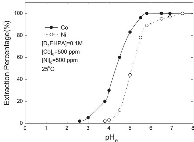
Fig. 2. Effect of  $\text{pH}_e$  on the extraction efficiencies of Co and Ni(II) in  $\text{H}_2\text{SO}_4$  using  $0.1 \text{ mol/dm}^3$   $\text{D}_2\text{EHPA}$ .
