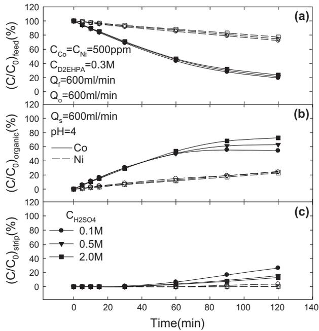
Fig. 5. Time profiles of the extraction and re-extraction for Co(II) and Ni(II) with D<sub>2</sub>EHPA in HFMCs at different strip acidity: (a) feed phase, (b) organic phase, and (c) strip phase.
