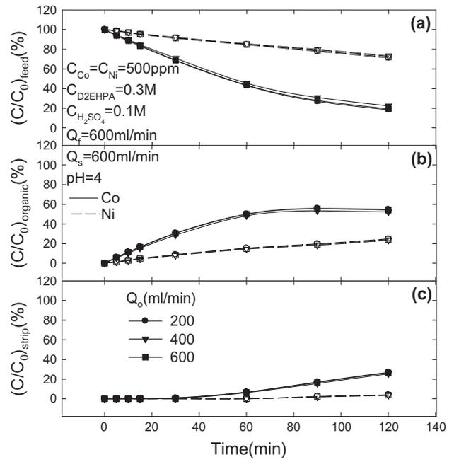
Fig. 7. Time profiles of extraction and re-extraction for Co(II) and Ni(II) in HFMCs at different flow rates of organic phase: (a) feed phase, (b) organic phase, and (c) strip phase.
