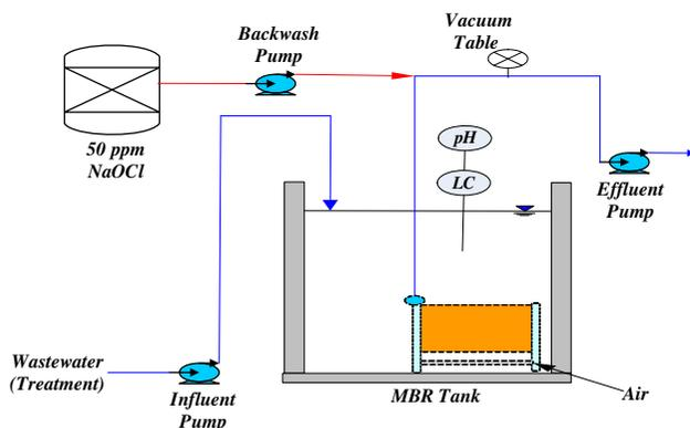
Fig. 1. Schematic diagram of the MBR pilot reactor.
