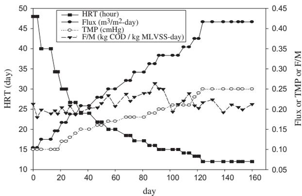
Fig. 4. Variation of operation parameters in the MBR system.
