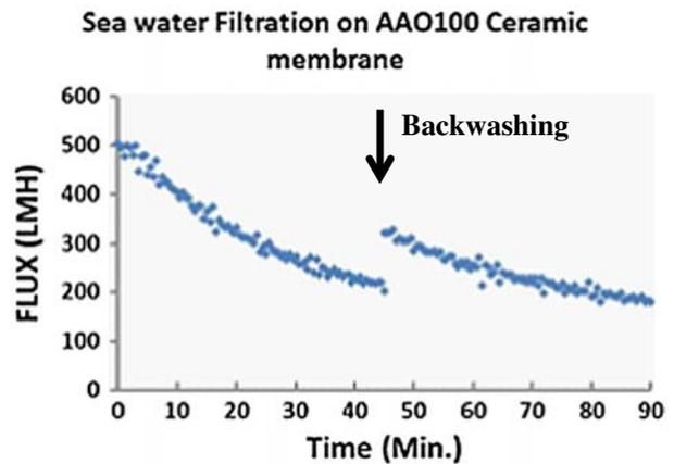
Fig. 8. Seawater filtration and BW.
