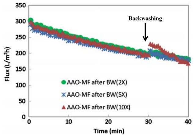
Fig. 11. Influence of BW flux on flux recovery (AAO100)–Seawater filtration.
