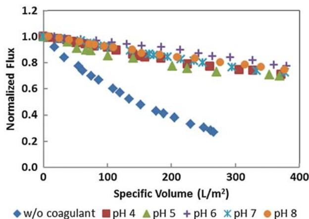
Fig. 14. Flux decline of AAO100 membranes at different pH conditions with 4 mg/l Fe coagulant.
