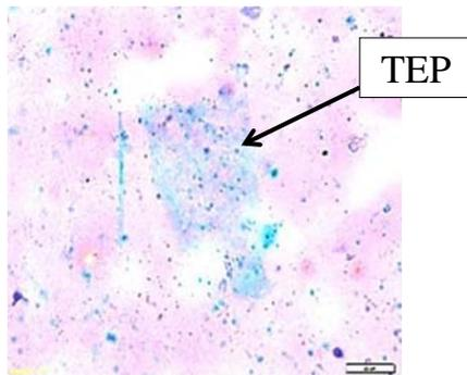
Fig. 9. TEP on AAO100 after Red Sea water filtration.
