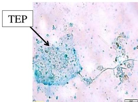
Fig. 10. TEP on AAO100 after BW with Milli Q water.
