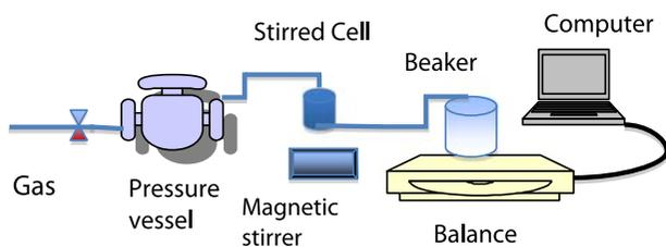
Fig. 2. Schematic layout of amicon stirred cell.
