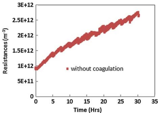
Fig. 7. Seawater filtered with monolith ceramic microfiltration system at constant flux of 150 LMH and BW interval of 2.5 h.
