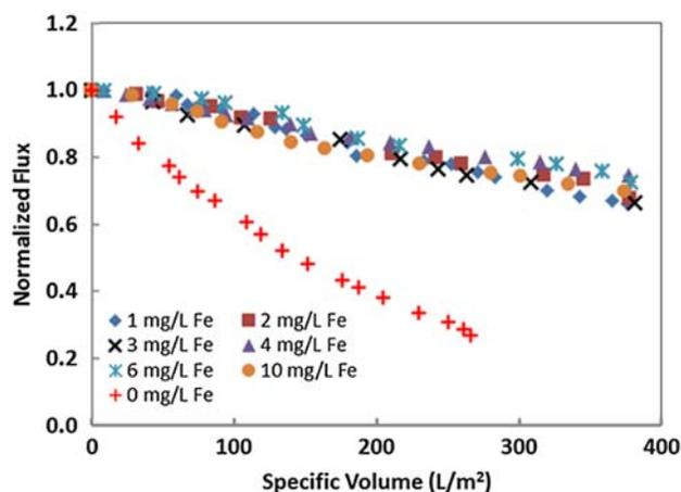
Fig. 13. Flux decline of AAO100 membranes at different coagulant doses—Seawater.
