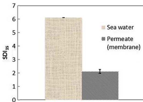
Fig. 3. Silt Density Index ( $\text{SDI}_{15}$ ) measured for feed water (sea) and permeate.
