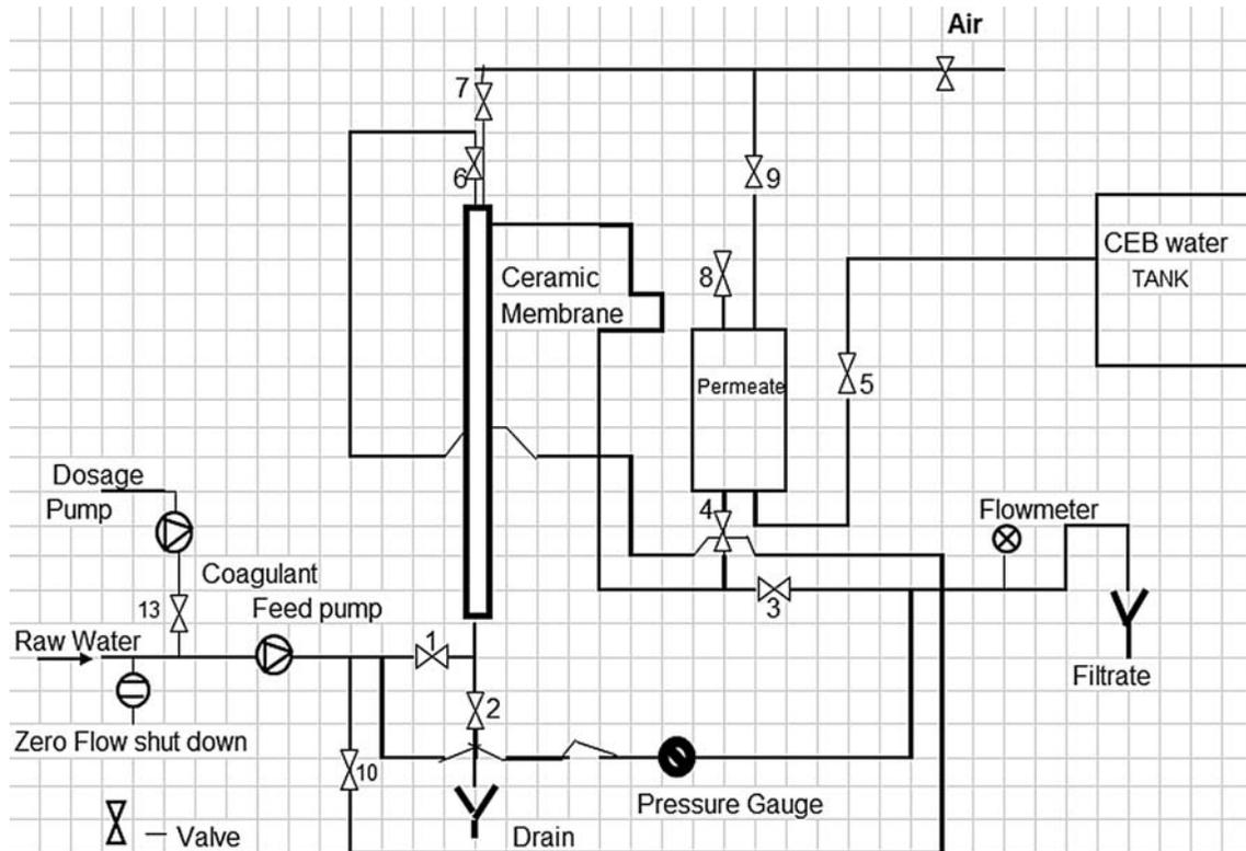
Fig. 1. Layout of the ceramic pilot plant.
