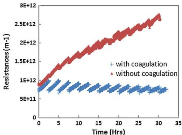
Fig. 15. Influence of coagulation (4 mg/L Fe) in reducing membrane fouling from seawater.
