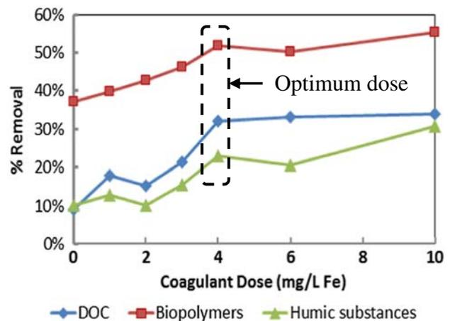
Fig. 12. High molecular weight NOM removal from ceramic anopore MF membrane (AAO100) at different coagulant doses ( $J_o \approx 500$  LMH)–Bench.
