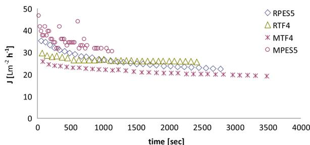
Fig. 1. Flux values of the hydrolysate and the model solution on different membranes. (Pressure: 0.35 MPa, temperature: 26 ± 0.5°C, 350 rpm, RPES5 – hydrolysate on PES5 membrane, RTF4 – hydrolysate on TF4 membrane, MTF4 – model solution on TF4 membrane, MPES5 – model solution on PES5 membrane).
