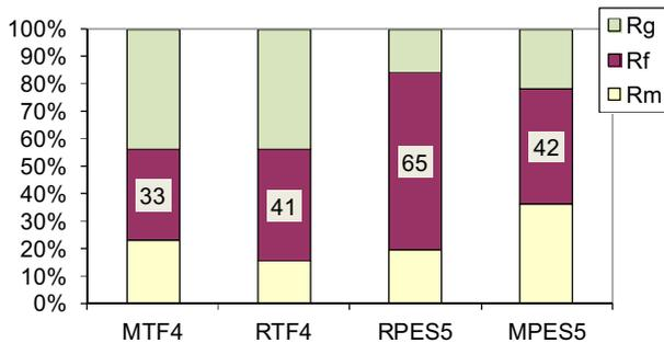
Fig. 2. Resistances of separation of model solution and hydrolysate with PES5 and TF4 membranes. (RTF4 – hydrolysate on TF4 membrane, MTF4 – model solution on TF4 membrane, RPES5 – hydrolysate on PES5 membrane, MPES5 – model solution on TF4 membrane,  $R_g$  – gel resistance,  $R_f$  – fouling resistance,  $R_m$  – membrane resistance).
