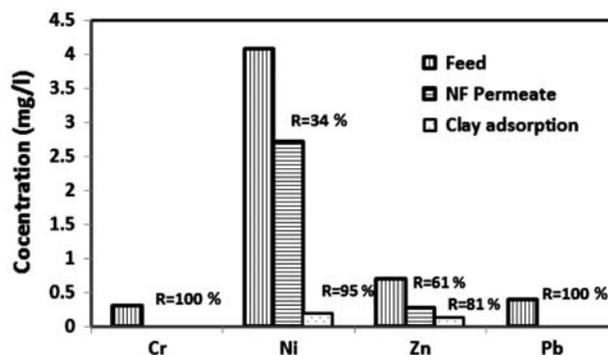
Fig. 7. Heavy metals concentrations after individual treatment processes for enriched STWW sample.
