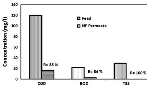
Fig. 3. COD, BOD, and TSS reduction after NF treatment for both typical and enriched STWW samples.
