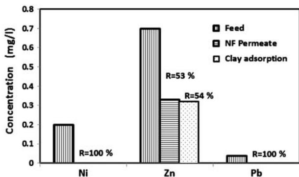
Fig. 6. Heavy metals concentrations after individual treatment processes for typical STWW sample.
