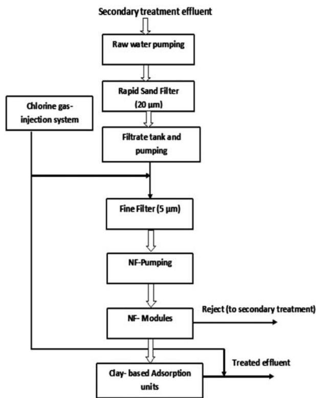
Fig. 8. Proposed NF/adsorption system for treatment of STWW.
