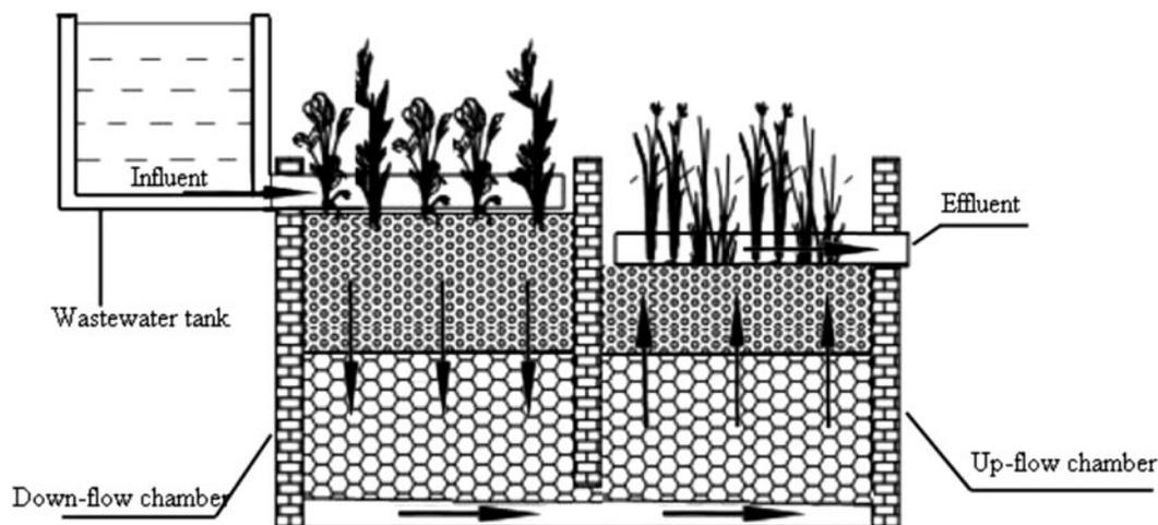
Fig. 1. Schematic of the IVCW mesocosm.
