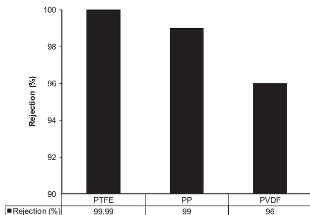
Fig. 3. Glucose rejection values of the applied membranes. ( $T_h = 65^\circ\text{C}$ ,  $Q_h = 600\text{ mL/min}$ ,  $C_i = 50\text{ kg/m}^3$ , and  $Q_s = 0.453\text{ Nm}^3/\text{h}$ ).
