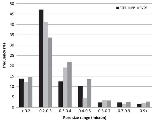
Fig. 2. Pore size distribution of applied membranes analyzed by AFM method. (PTFE, PP, and PVDF with 0.22  $\mu\text{m}$  reported pore size).
