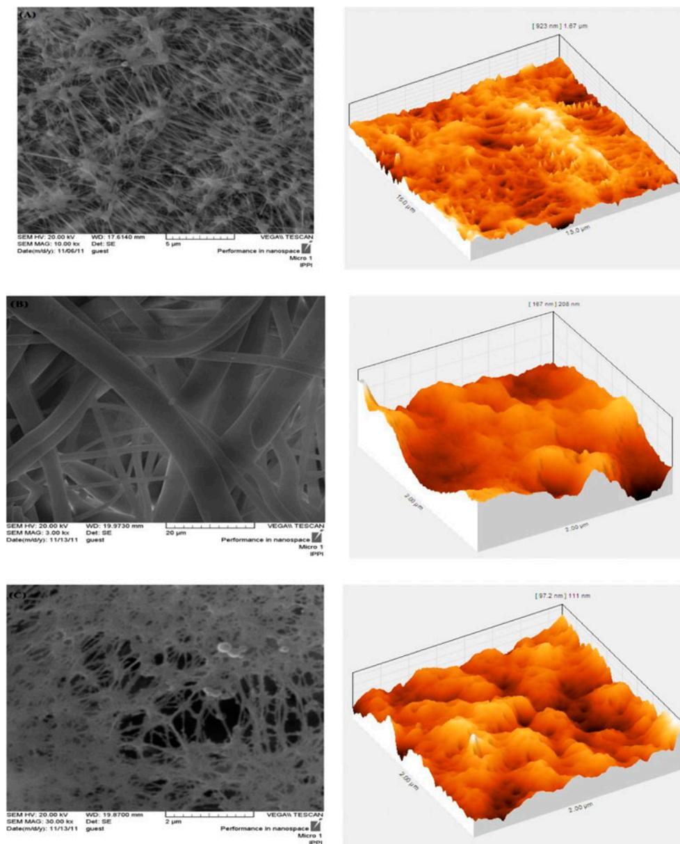
Fig. 1. SEM (left) and AFM (right) images of (A) PTFE, (B) PP, and (C) PVDF membranes with  $0.22\mu\text{m}$  reported pore size.
