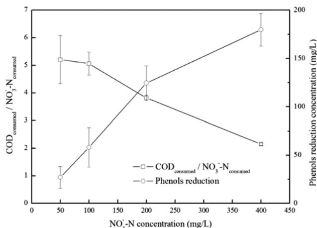
Fig. 6. Reduction of phenols and ratio of  $\text{COD}_{\text{consumed}} / \text{NO}_3^-$ -N<sub>consumed</sub> under different influent  $\text{NO}_3^-$ -N concentrations in the ANMBBR.
