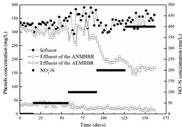
Fig. 2. Evolution of phenols in the influent of ANMBBR and effluent of ANMBBR and AEMBBR at different NO<sub>3</sub><sup>-</sup>-N concentrations.
