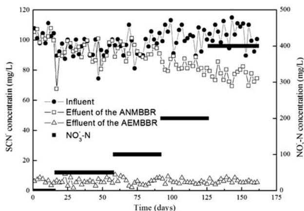
Fig. 3. Evolution of  $\text{SCN}^-$  in the influent of the ANMBBR and effluent of the ANMBBR and AEMBBR at different  $\text{NO}_3^-$ -N concentrations.
