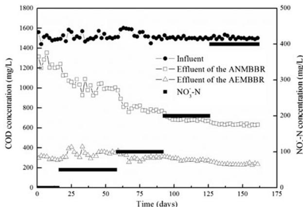
Fig. 1. Evolution of COD in the influent of the ANMBBR and effluent of the ANMBBR and AEMBBR at different NO<sub>3</sub><sup>-</sup>-N concentrations.
