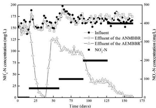
Fig. 4. Evolution of  $\text{NH}_4^+$ -N in the influent of the ANMBBR and effluent of the ANMBBR and AEMBBR at different  $\text{NO}_3^-$ -N concentrations.
