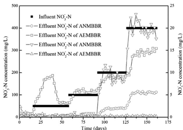
Fig. 5. Evolution of  $\text{NO}_2^-$ -N and  $\text{NO}_3^-$ -N in the effluent of the ANMBBR and AEMBBR at different  $\text{NO}_3^-$ -N concentrations.
