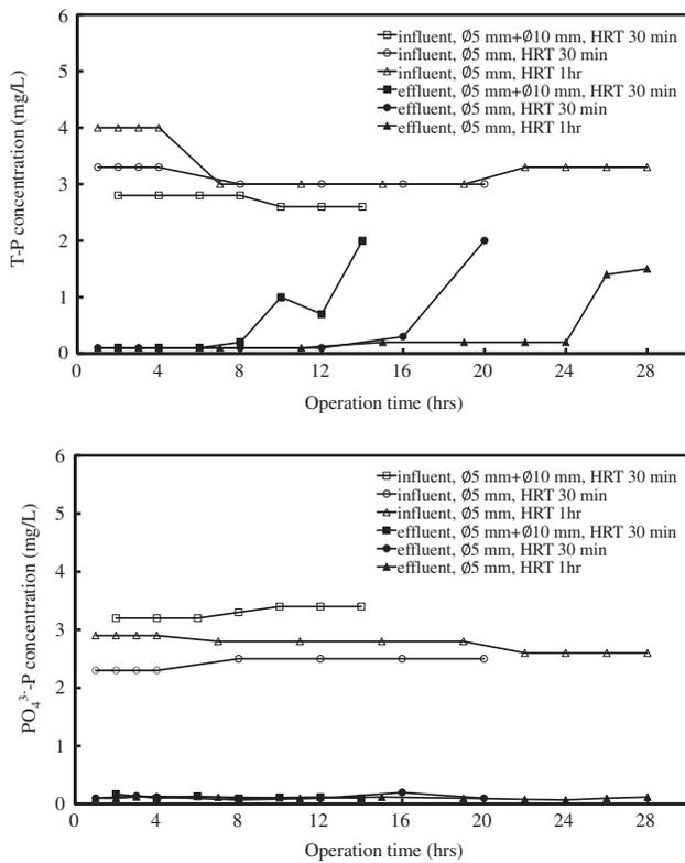
Fig. 12. T-P and S-P concentrations of influent and effluent of filter bed with chemical treatment.
