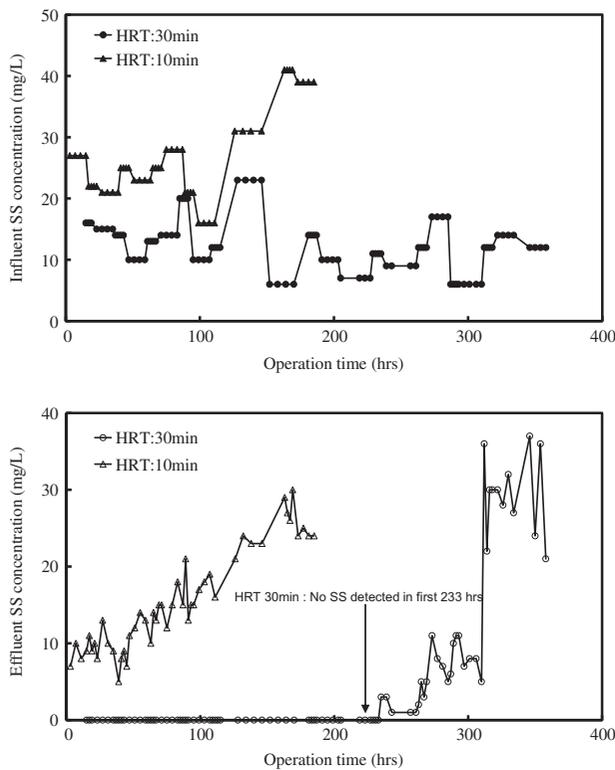
Fig. 6. SS concentrations of influent and effluent to the changes of filter bed HRT (Type-I cage packed with  $\varnothing 5$  mm tubes).
