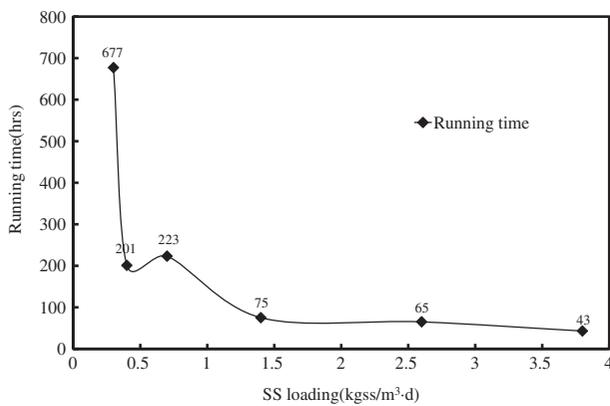
Fig. 9. Variations of running time to the changes of SS loading rate of filter bed for advanced SS treatment.
