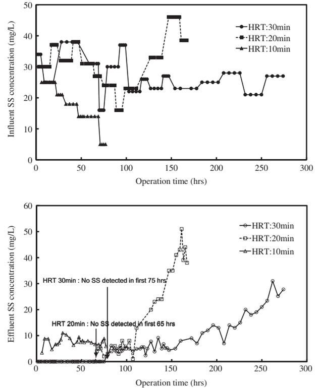
Fig. 7. SS concentrations of influent and effluent to the changes of filter bed HRT (Type-II cage packed with  $\varnothing 5$  mm tubes).
