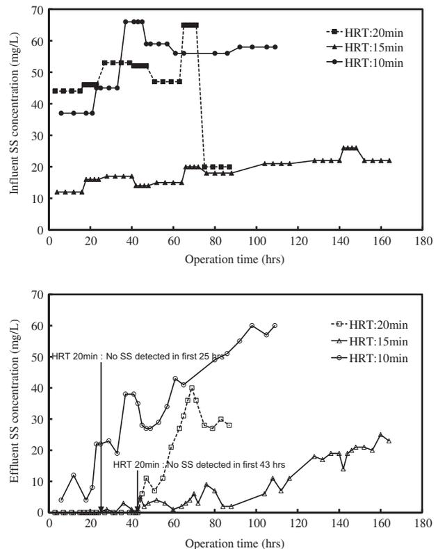
Fig. 8. SS concentrations of influent and effluent to the changes of filter bed HRT (Type-II cage packed with  $\varnothing 3$  mm tubes).
