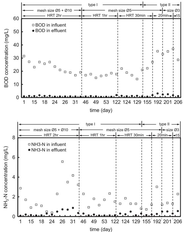
Fig. 11. BOD and  $\text{NH}_3\text{-N}$  concentrations of influent and effluent of filter bed.
