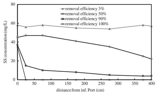
Fig. 14. Variations of SS concentration over the length of filter bed to the changes of SS removal efficiency.
