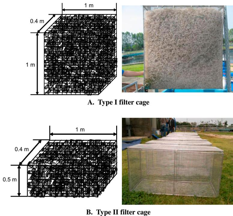
Fig. 4. Filter cage packed with meshed filter tubes.
