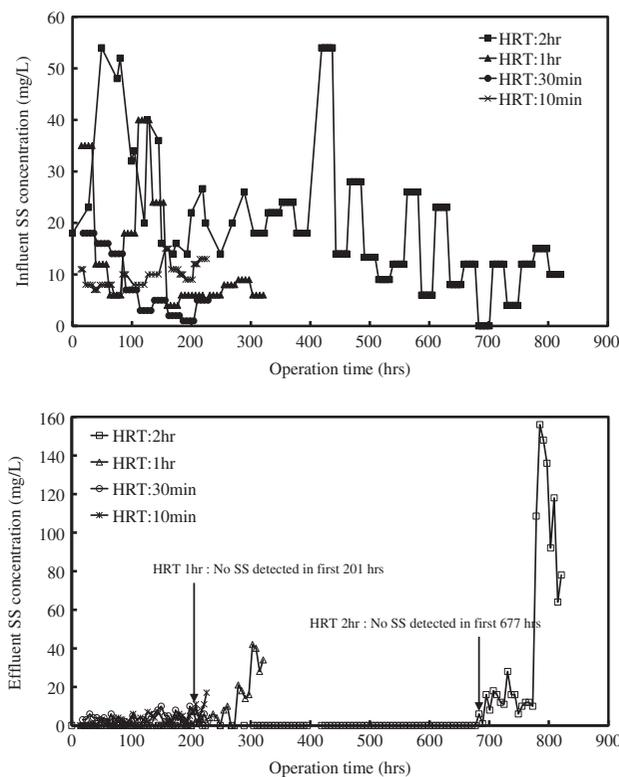
Fig. 5. SS concentrations of influent and effluent to the changes of filter bed HRT (Type-I cage packed with ∅5 mm + ∅10 mm tubes).
