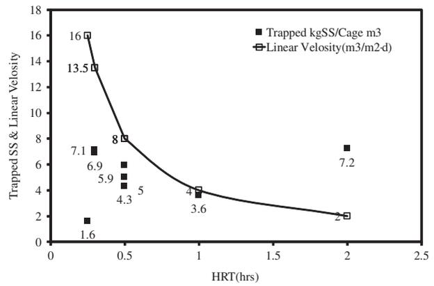
Fig. 10. Results of linear velocity and trapped mass of SS per tube cage volume to the changes of HRTs of filter bed.
