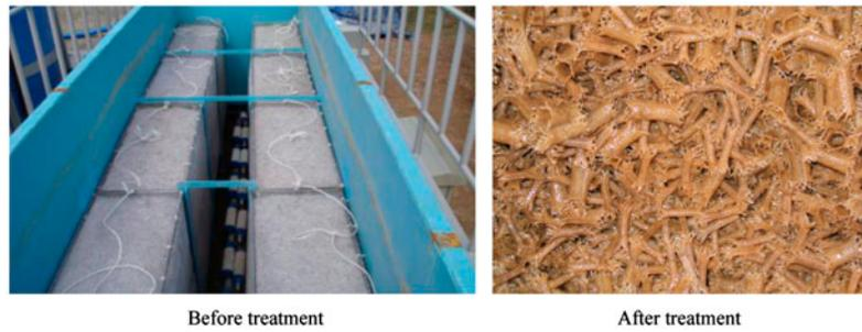
Fig. 3. Filter bed of pilot plant equipped with meshed tubes.
