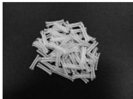
Fig. 1. Meshed synthetic fiber tubes.
