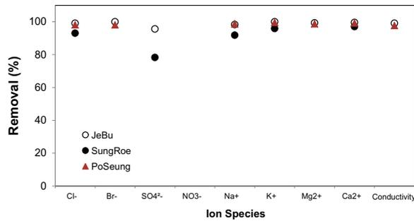
Fig. 2. Ion removal (%) by the ED in the laboratory system.
