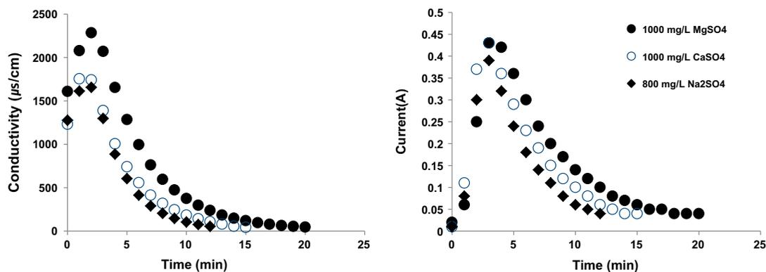
Fig. 7. Changes in conductivity and currents at 12 V with  $\text{MgSO}_4$ ,  $\text{CaSO}_4$ ,  $\text{Na}_2\text{SO}_4$  solution of 1,000, 1,000, and 800 mg/L.
