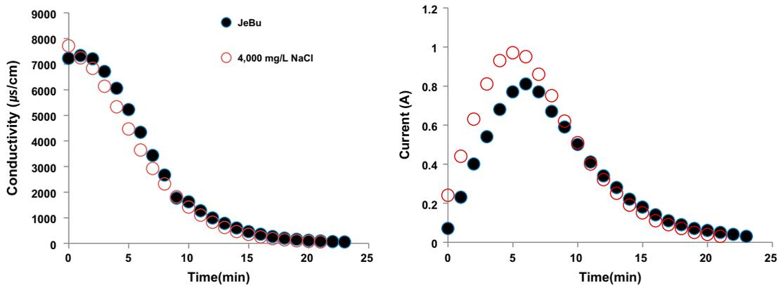
Fig. 4. Changes in conductivity and currents at 12 V with JeBu groundwater and NaCl solution of 4,000 mg/L.
