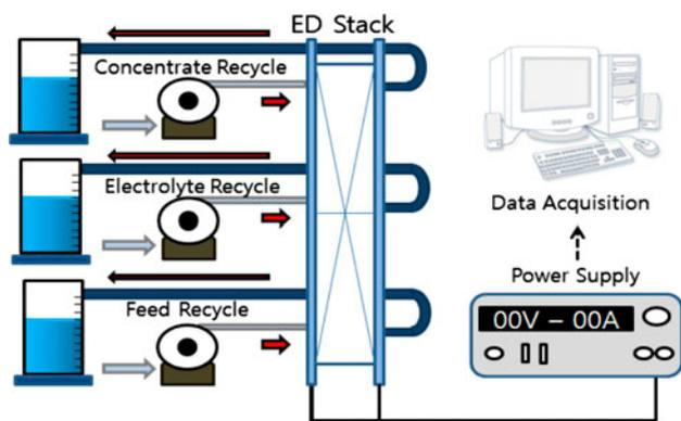
Fig. 1. Scheme of ED system in this study.
