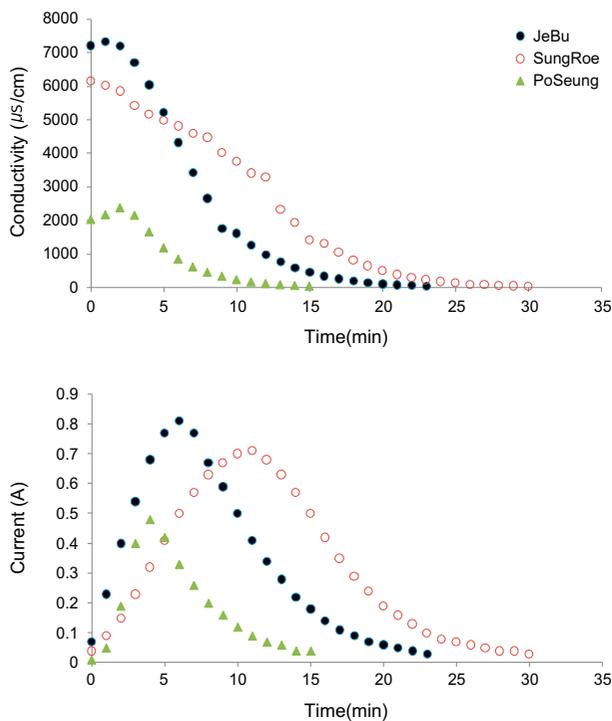
Fig. 3. Changes in conductivity and current during a batch mode of ED with a constant voltage operation (i.e. 12 V).
