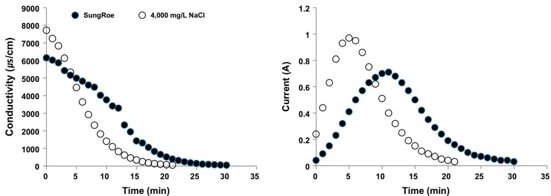
Fig. 5. Changes in conductivity and currents at 12 V with SungRoe groundwater and NaCl solution of 4,000 mg/L.
