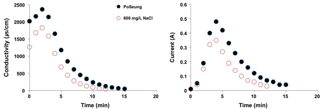
Fig. 6. Changes in conductivity and currents at 12 V with PoSeung groundwater and NaCl solution of 600 mg/L.
