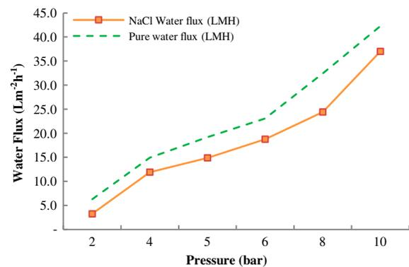
Fig. 4. Water permeability as a function of the applied pressure.
