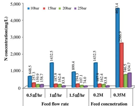
Fig. 8. Predicted N concentration in the NF permeate using the diluted SOA (DS) as FS.
