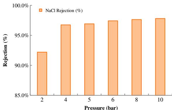
Fig. 5. Effects of applied pressure on NaCl rejection for the initial investigation.
