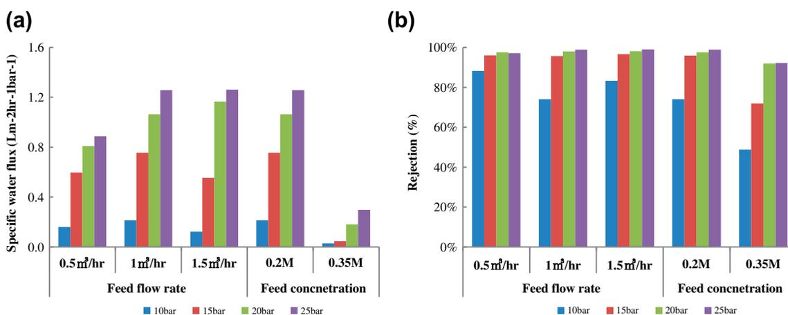
Fig. 6. Specific water flux (a) and rejection (b) with applied pressure for the diluted fertilizer (SOA) as FS for NF process at both different flow rate and concentration.
