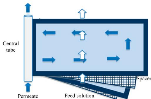
Fig. 2. Flows in NE90 spiral-wound membrane.
