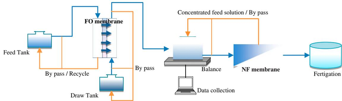
Fig. 3. Schematic diagram of pilot-scale FDFO-NF desalination process.
