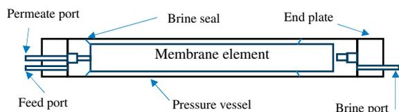
Fig. 1. Pressure vessel with NF membrane element.
