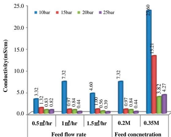
Fig. 7. Final permeate water flux conductivity of pilot-scale NF process at applied pressures.
