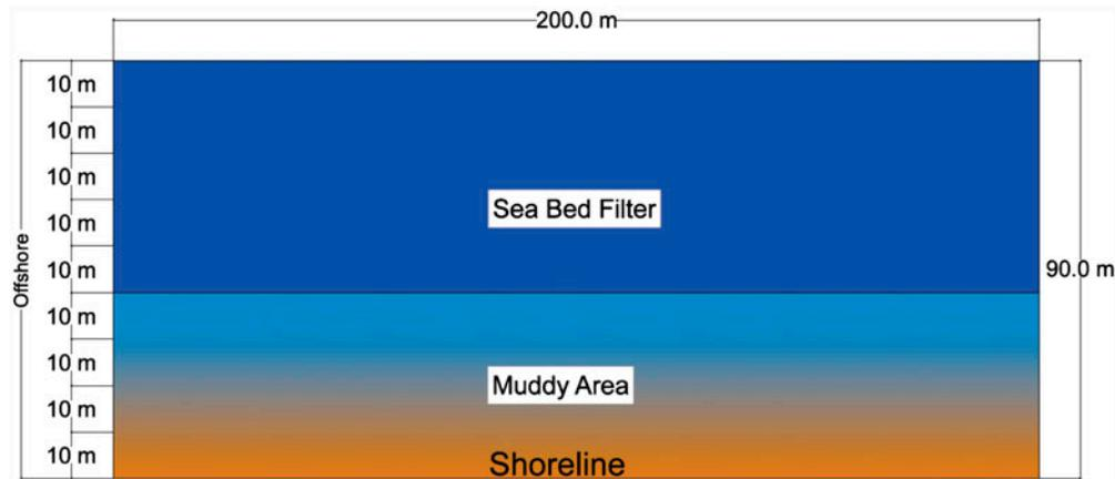
Fig. 5. The location of the seabed gallery cells should be located offshore of the muddy sediment area to avoid mud infiltration. This is about 40 m seaward of the shoreline.
