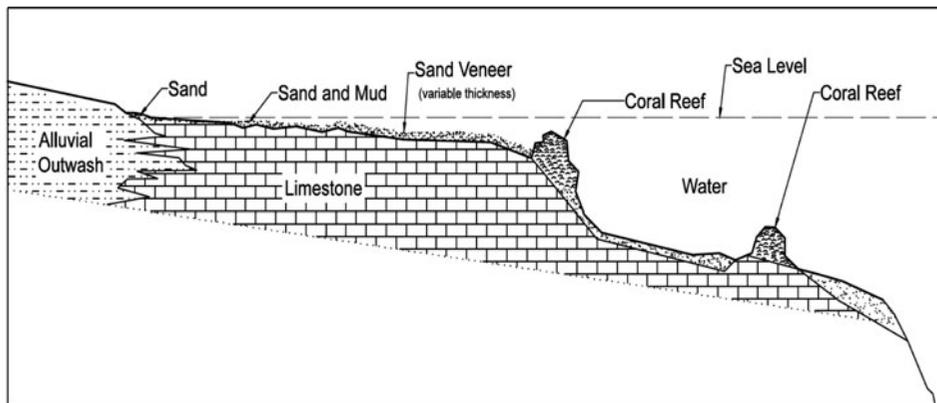
Fig. 3. The nearshore area can be classified as an arid carbonate rimmed shelf capped with a predominately carbonate sand veneer with some “patches” of muddy sand.
