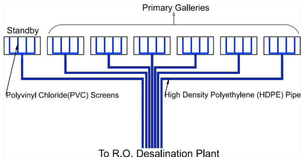
Fig. 7. Preliminary conceptual design of the expansion plan for KAEC seabed.
