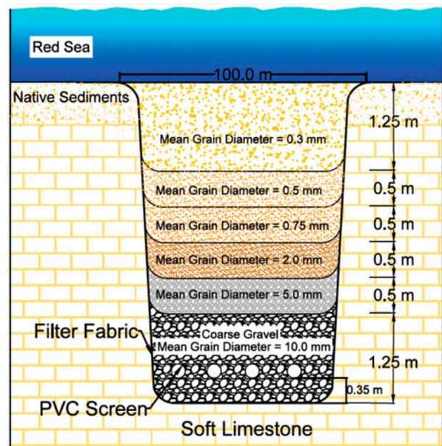
Fig. 6. Preliminary design of the KAEC seabed gallery.
