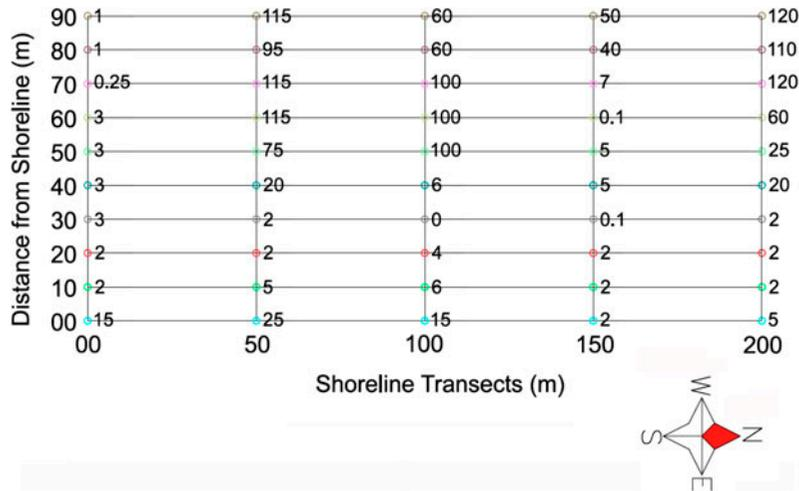
Fig. 2. Sampling grid at the KAEC showing the thickness of sand in centimeters.
