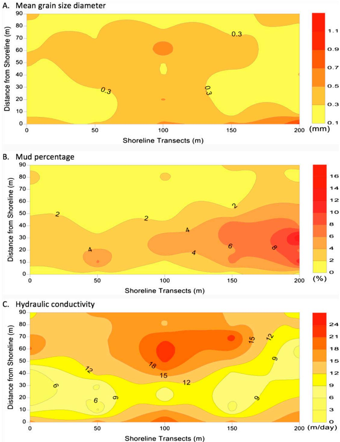
Fig. 4. Sediment grain size characteristics and hydraulic conductivity within the study area at the KAEC site.
