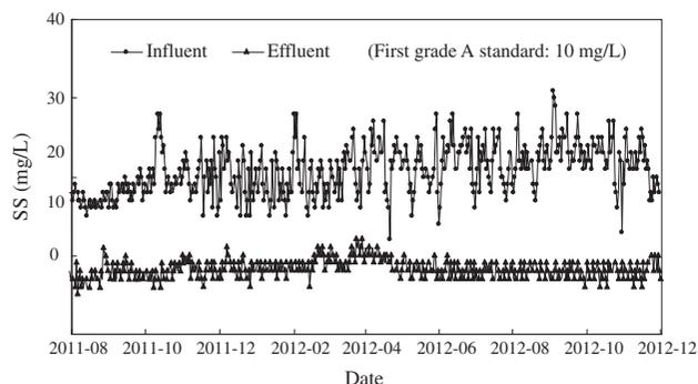
Fig. 3. The removal of SS during the micro-flocculation and sand filtration process.
