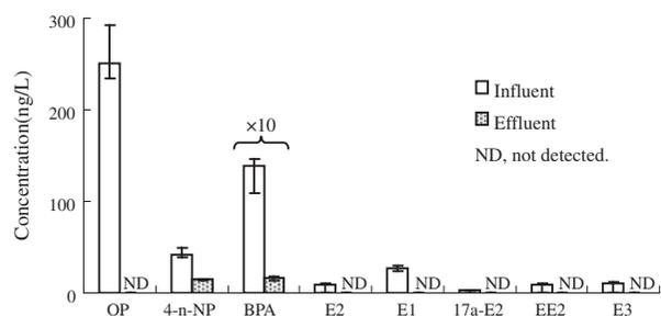
Fig. 6. Removal of EDCs during micro-flocculation and sand filtration.
