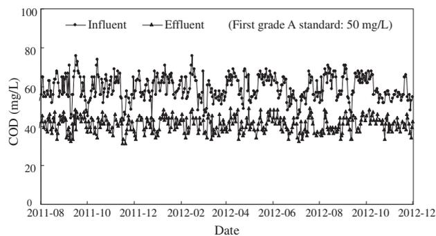
Fig. 4. The removal of COD during the micro-flocculation and sand filtration process.
