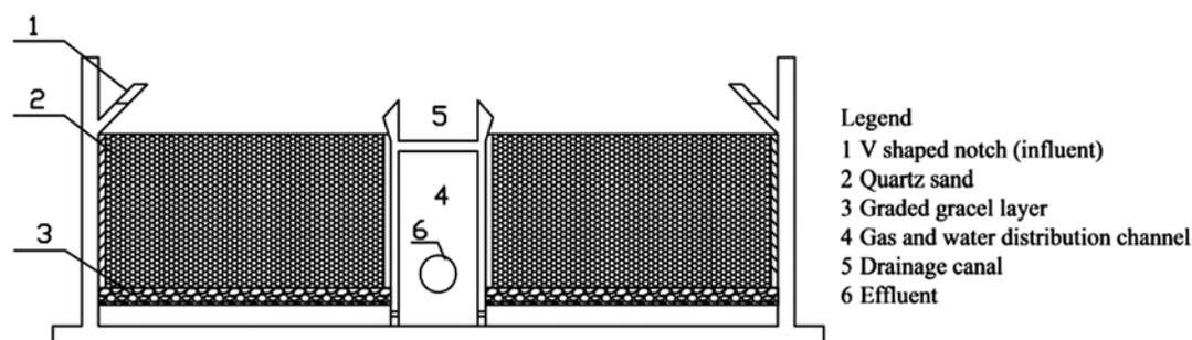
Fig. 1. Schematic representation of the micro-flocculation and sand filtration tank.
