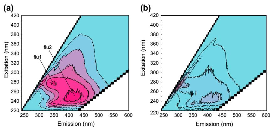
Fig. 5. EEM spectra before (a) and after (b) the micro-flocculation and sand filtration process.
