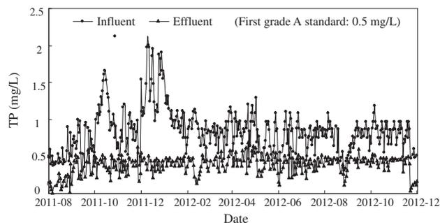
Fig. 2. The removal of TP during the micro-flocculation and sand filtration process.
