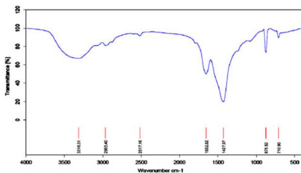
Fig. 2. FTIR spectrum of eggshell membrane.
