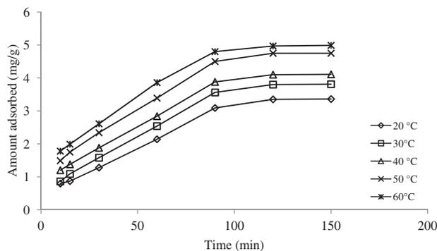
Fig. 5. Effect of temperature on the Cr (VI) ions uptake by eggshell membrane at pH 4 [Cr (VI) ion concentration = 5 mg/l, dosage of sorbent = 3.5 g, contact time = 15, 30, 60, 90, 120, and 150 min].
