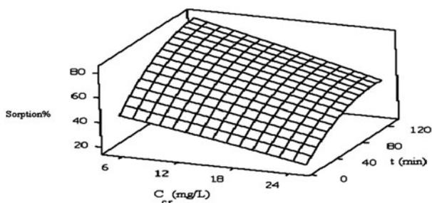
Fig. 7. Response surface of the percentage sorption of Cr (VI) ions versus Cr(VI) ions concentration and contact time at 20°C [dosage of sorbent = 3.78 g, pH = 3.54].
