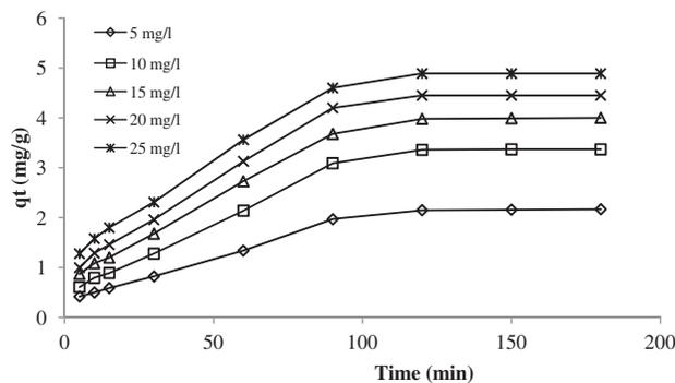
Fig. 4. Effect of contact time on the Cr(VI) ions uptake over eggshell membrane at 20°C [Cr(VI) ion concentration = 5 to 25 mg/L, sorbent dosage = 3.5 g and pH = 4].
