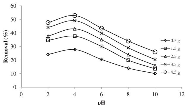
Fig. 3. Effect of pH on the removal of Cr(VI) ions by eggshell membrane at 20°C [Cr(VI) concentration = 5 mg/L, contact time = 60 min, sorbent dosage = 0.5 to 4.5 g].
