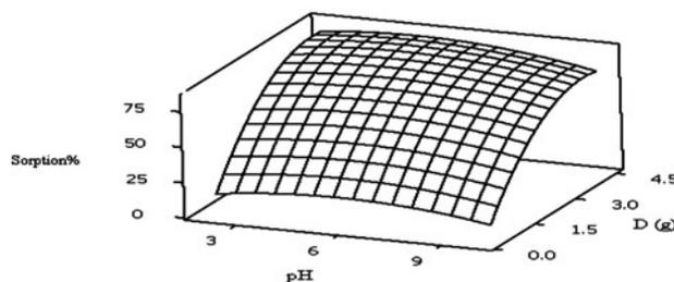
Fig. 8. Response surface of the percentage sorption of Cr (VI) ions versus pH and dosage of sorbent at 20°C [contact time = 117.52, Cr(VI) ion concentration = 5.0 mg/L].
