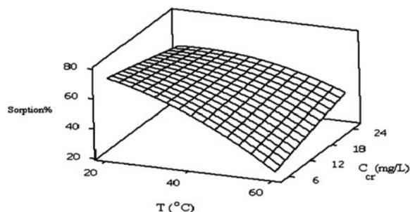
Fig. 6. Response surface of the percentage sorption of Cr (VI) ions versus temperature and Cr(VI) ion concentration [dosage of sorbent = 3.78 g, contact time = 117.52 min, pH = 3.54].
