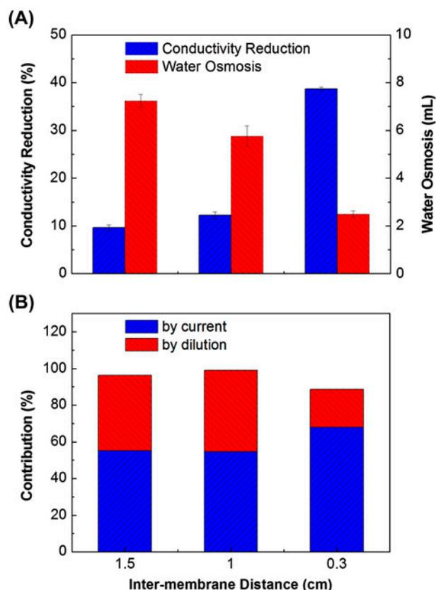
Fig. 7. The desalination performance of the MDC with different inter-membrane distances at the same HRT of 6 h: (A) conductivity reduction (blue) and the amount of water osmosis (red); and (B) The contributions to conductivity reduction by electric current (blue) and dilution (red). (For interpretation of the references to color in this figure legend, the reader is referred to the web version of this article.)
