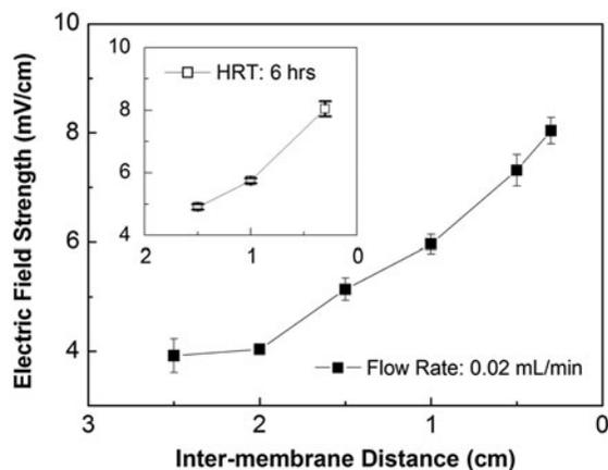
Fig. 4. The electric field strength at different inter-membrane distances when the salt feeding rate was same at 0.02 mL/min. Inset figure: the electric field strength with 0.3, 1.0, and 1.5 cm inter-membrane distance at the same HRT of 6 h. Note: electric field strength was calculated based on the distance between the anode and the cathode electrodes, instead of the inter-membrane distance.
