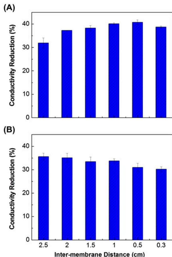
Fig. 2. The conductivity reduction of the salt solution at different inter-membrane distances at two different initial salt concentrations: (A) 10 g/L; and (B) 30 g/L.
