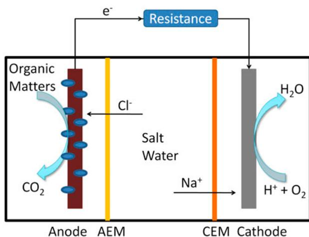
Fig. 1. The schematic of a MDC. AEM: anion exchange membrane; CEM: cation exchange membrane.
