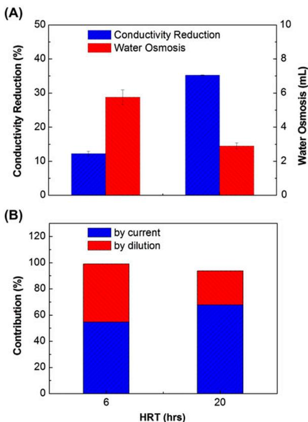
Fig. 8. The desalination performance of the MDC with same inter-membrane distance of 1 cm at two different HRTs of 6 and 20 h: (A) conductivity reduction (blue) and the amount of water osmosis (red); and (B) The contributions to conductivity reduction by electric current (blue) and dilution (red). (For interpretation of the references to color in this figure legend, the reader is referred to the web version of this article.)
