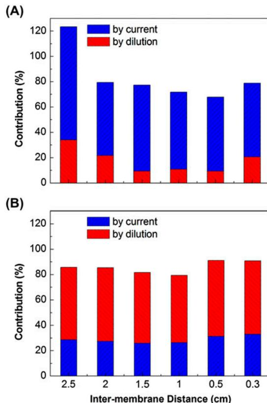
Fig. 5. The contributions to conductivity reduction by electric current (blue) and dilution (red) at two different initial salt concentrations: (A) 10 g/L; and (B) 30 g/L. (For interpretation of the references to color in this figure legend, the reader is referred to the web version of this article.)
