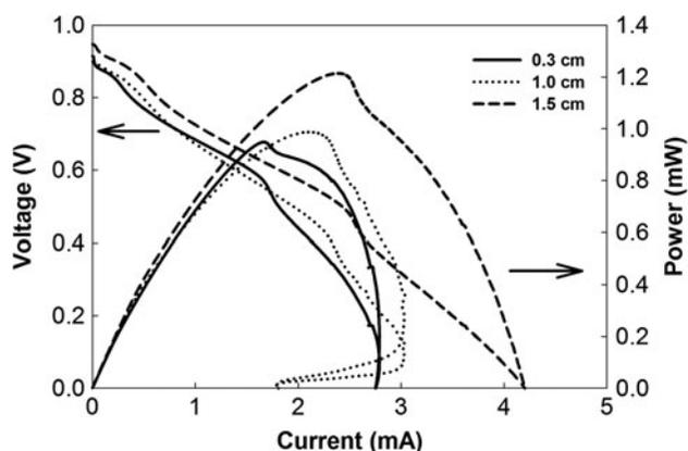
Fig. 6. The polarization curves (power and voltage vs. current) of the MDC with 0.3, 1.0, and 1.5 cm inter-membrane distance at the same HRT of 6 h.
