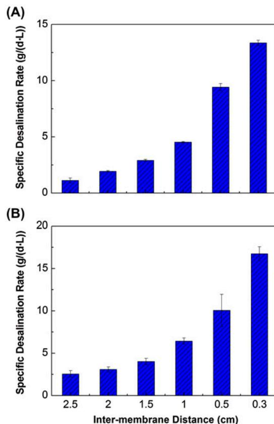
Fig. 3. The SDR at different inter-membrane distances at two different initial salt concentrations: (A) 10 g/L; and (B) 30 g/L.
