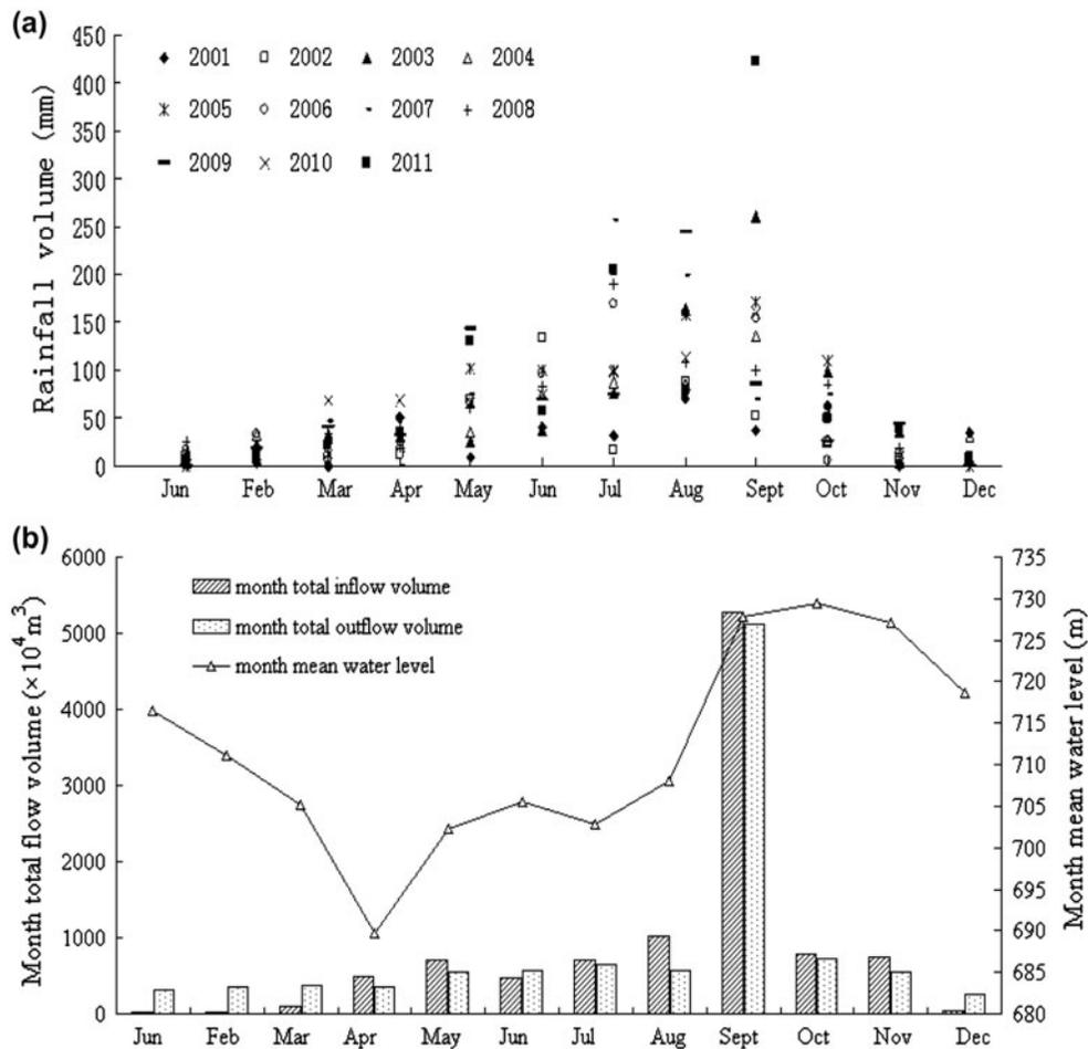
Fig. 4. Monthly rainfall changes in Shibiyanu reservoir from 2001 to 2011 (a), and variation of monthly total inflow volume, monthly total outflow volume, and water level in 2011 (b).
