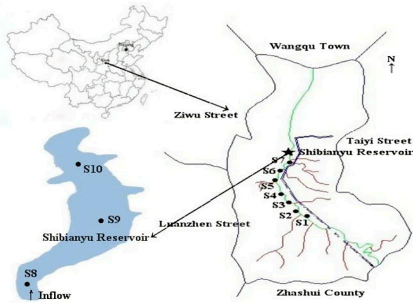
Fig. 1. Illustration of Shibiyanu reservoir showing the location of sampling and monitoring sites : S1–S7 are located in the upstream of Shibiyanu reservoir. S8, S9, and S10 are located in the river area, transition area, and deep water area of the reservoir, respectively.
