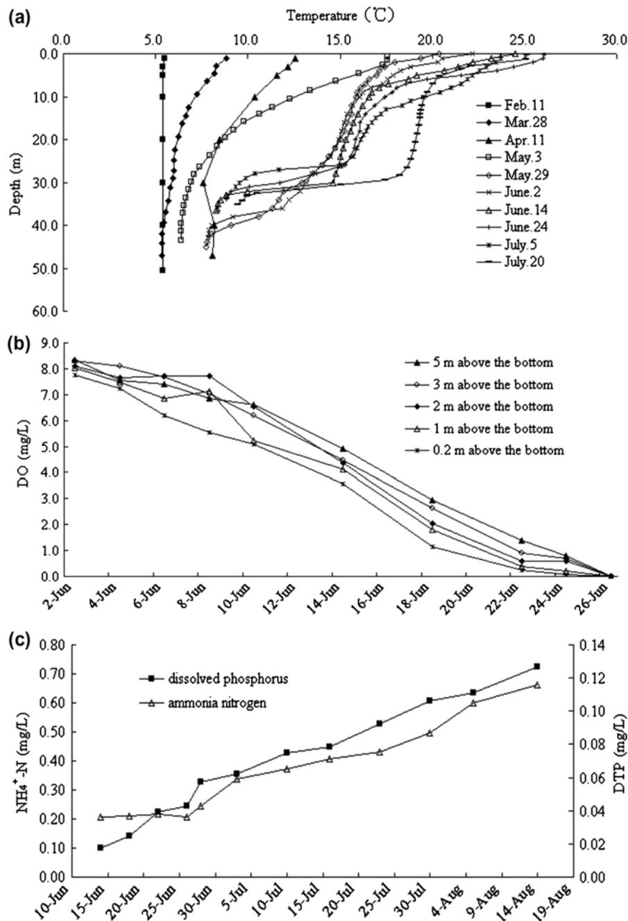
Fig. 3. Water temperature vertical distribution characteristics (a), DO concentration depletion in hypolimnion (b) and dynamic characteristic of ammonia nitrogen and dissolved phosphorus in overlying water above 0.2m of sediment in S10 (the deepest point of Shibiyanu reservoir).
