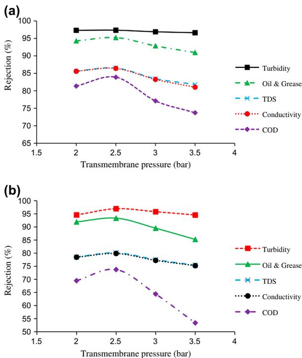
Fig. 5. Effect of TMP on pollutants removal at  $T=20^{\circ}\text{C}$  and (a)  $[\text{LAS}]=2\text{ mM}$ , (b)  $[\text{SDS}]=9\text{ mM}$ .
