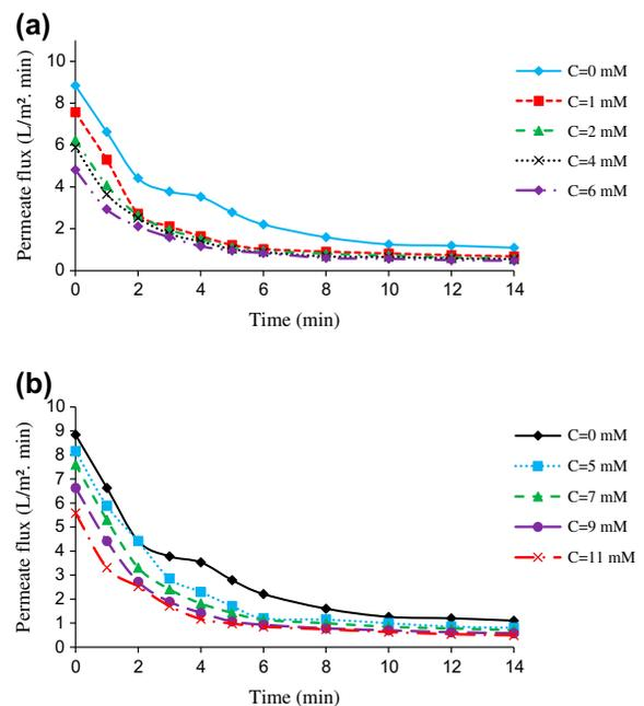
Fig. 2. Effect of surfactant concentration on permeate flux at  $T = 20^\circ\text{C}$  and  $\text{TMP} = 2.5 \text{ bar}$ : (a) LAS, (b) SDS.
