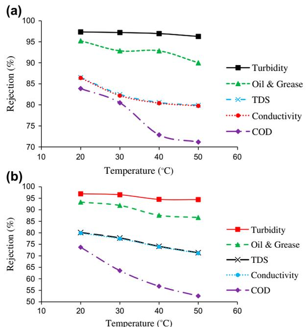
Fig. 7. Effect of temperature on pollutants removal at  $\text{TMP}=2.5\text{ bar}$  and (a)  $[\text{LAS}]=2\text{ mM}$ , (b)  $[\text{SDS}]=9\text{ mM}$ .
