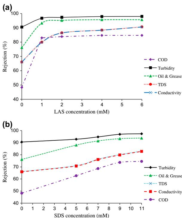
Fig. 3. Effect of surfactant concentration on pollutants removal at  $T=20^{\circ}\text{C}$  and  $\text{TMP}=2.5$  bar: (a) LAS, (b) SDS.
