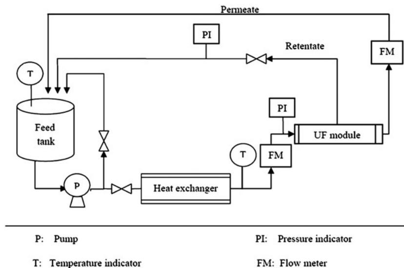
Fig. 1. Membrane pilot plant.
