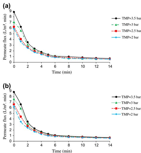
Fig. 4. Effect of TMP on Permeate flux at  $T=20^{\circ}\text{C}$  and (a) [LAS]=2 mM, (b) [SDS]=9 mM.
