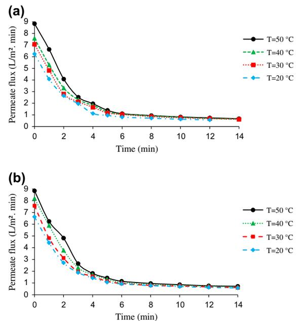
Fig. 6. Effect of temperature on Permeate flux at  $\text{TMP}=2.5\text{ bar}$  and (a)  $[\text{LAS}]=2\text{ mM}$ , (b)  $[\text{SDS}]=9\text{ mM}$ .
