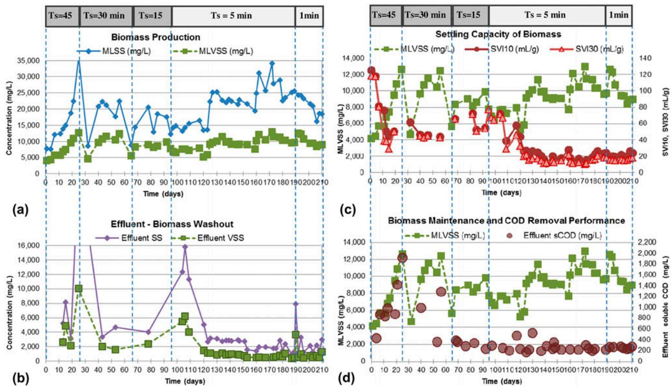
Fig. 2. Long-term monitoring for determining the impact of gradually decreased  $T_s$ : (a) biomass production (MLSS and MLVSS), (b) biomass washout (SS and VSS in the effluent), (c) settling properties (MLVSS and SVI), and (d) COD removal (soluble COD in the effluent).
