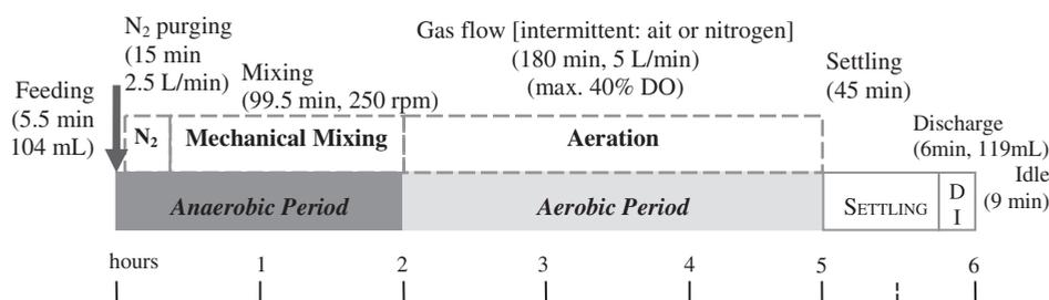
Fig. 1. Cycle configuration during start-up (days 1–25).
