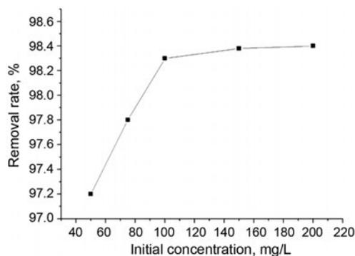
Fig. 4. Effect of initial concentration on adsorption (solid to liquid ratio 2.5 mg/L, 60°C, pH 7).
