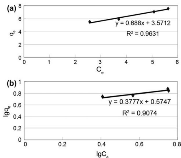
Fig. 6. Adsorption isotherm fitting (60°C, 5 h, solid to liquid ratio 2.5 g/L): (a) Langmuir model; (b) Freundlich model.
