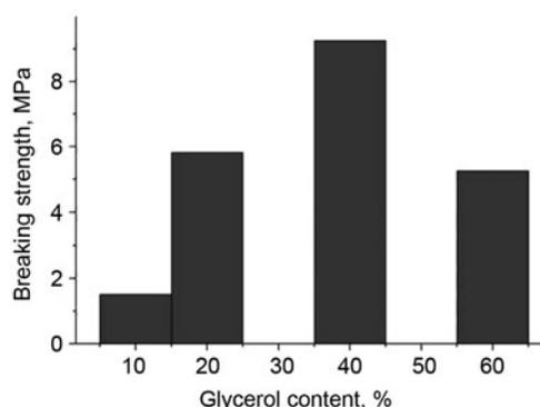
Fig. 1. Effect of glycerol content on breaking strength (glycerol content 160°C, 5 MPa, 3 min).
