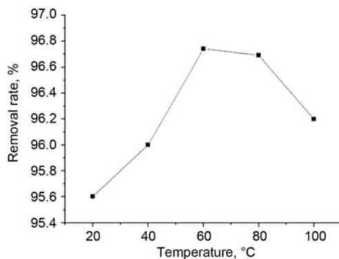
Fig. 2. Effect of temperature on adsorption (initial concentration 100 mg/L, solid to liquid ratio 12.5 mg/L, pH 7).
