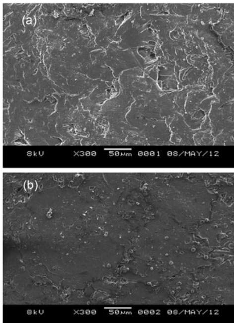
Fig. 7. SEM pictures of keratin film (a) before and (b) after adsorption.
