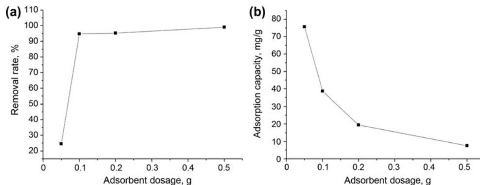
Fig. 3. Effect of adsorbent dosage on adsorption (initial concentration 100 mg/L, 60°C, 40 mL, pH 7): (a) effect of adsorbent dosage on removal rate; (b) effect of adsorbent dosage on removal rate.
