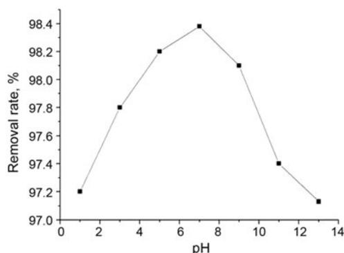
Fig. 5. Effect of pH on adsorption (solid to liquid ratio 2.5 mg/L, 60°C, 100 mg/L).
