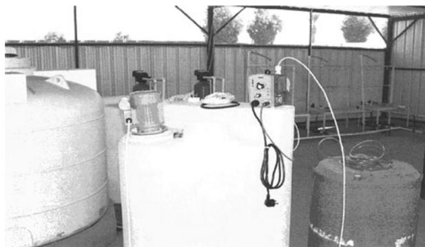
Fig. 5. Pumping of hydrogen sulfide-spiked groundwater to the treatment units at Mishref site.
