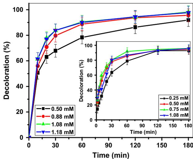
Fig. 2. Effect of HP and SPS (inset) dosage on the decoloration of AB 29: [Fe $^{2+}$ ] = 0.015 mM, [AB 29] = 0.07 mM, and pH = 3.
