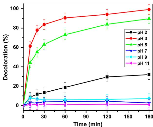
Fig. 3. Effect of pH on the decoloration of AB 29 in  $\text{Fe}^{2+}/\text{HP}$  system:  $[\text{HP}] = 1.08 \text{ mM}$ ,  $[\text{Fe}^{2+}] = 0.015 \text{ mM}$ ,  $[\text{AB 29}] = 0.07 \text{ mM}$ .
