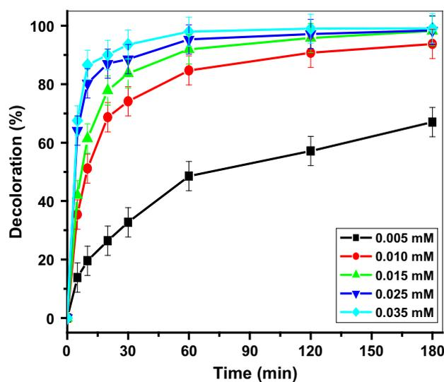
Fig. 5. Effect of  $[\text{Fe}^{2+}]$  on the decoloration of AB 29 in  $\text{Fe}^{2+}/\text{HP}$  system:  $\text{pH} = 3$ ,  $[\text{HP}] = 1.08 \text{ mM}$ , and  $[\text{AB 29}] = 0.07 \text{ mM}$ .
