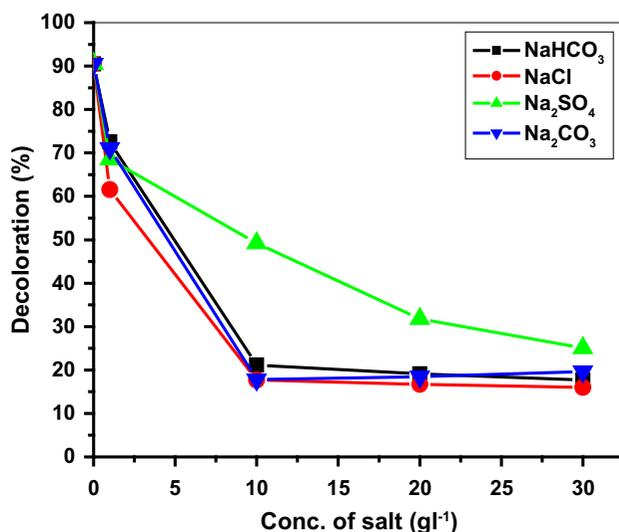
Fig. 7. Effect of inorganic ions on the decoloration of AB 29 by Fe<sup>2+</sup>/HP system: [AB 29]=0.07 mM, pH=3, [Fe<sup>2+</sup>]=0.015 mM, [HP]=1.08 mM, and Reaction time = 60 min.
