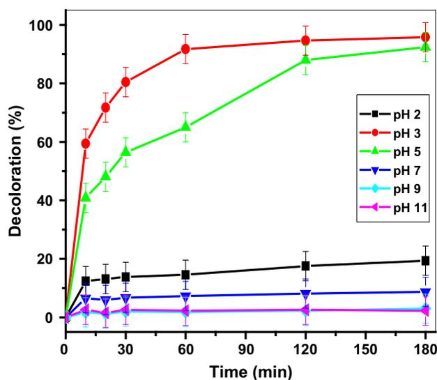
Fig. 4. Effect of pH on the decoloration of AB 29 in  $\text{Fe}^{2+}/\text{SPS}$  system:  $[\text{SPS}] = 0.75 \text{ mM}$ ,  $[\text{Fe}^{2+}] = 0.015 \text{ mM}$ ,  $[\text{AB 29}] = 0.07 \text{ mM}$ .
