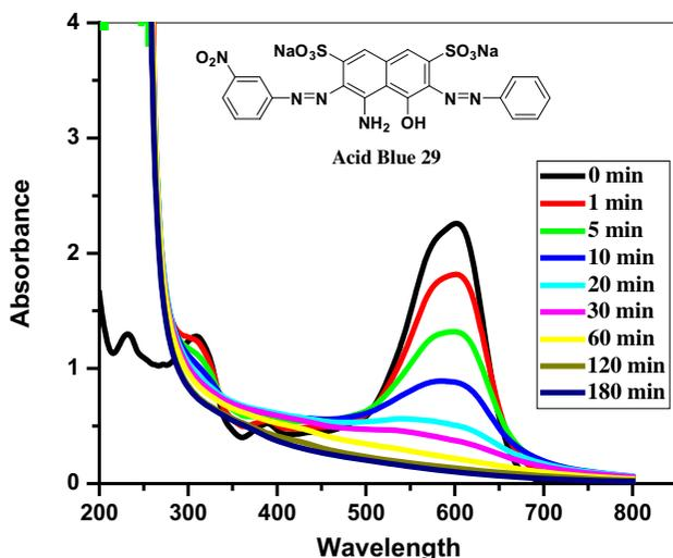
Fig. 1. UV–vis spectral changes of AB 29 in  $Fe^{2+}/HP$  system:  $[HP] = 1.08 \text{ mM}$ ,  $[Fe^{2+}] = 0.015 \text{ mM}$ ,  $[AB \ 29] = 0.07 \text{ mM}$ , and  $pH = 3$ . Inset: Structure of AB 29.
