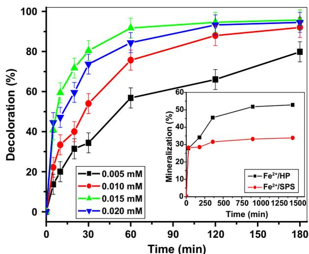
Fig. 6. Effect of  $[\text{Fe}^{2+}]$  on the decoloration of AB 29 in  $\text{Fe}^{2+}$ /SPS system: pH = 3, [SPS] = 0.75 mM, [AB 29] = 0.07 mM. In set: Mineralization of AB 29 at pH 3: [AB 29] = 0.07 mM,  $[\text{Fe}^{2+}]$  = 0.015 mM, [HP] = 1.08 mM, and [SPS] = 0.75 mM.
