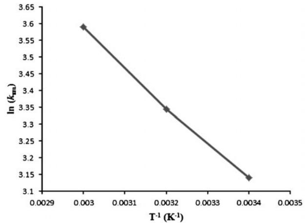
Fig. 10. plot of  $\ln k_{sm}$  vs.  $T^{-1}$ : estimation of the activation energy,  $E_a$ , for the dsorption of silver ion onto PAN-TETA.
