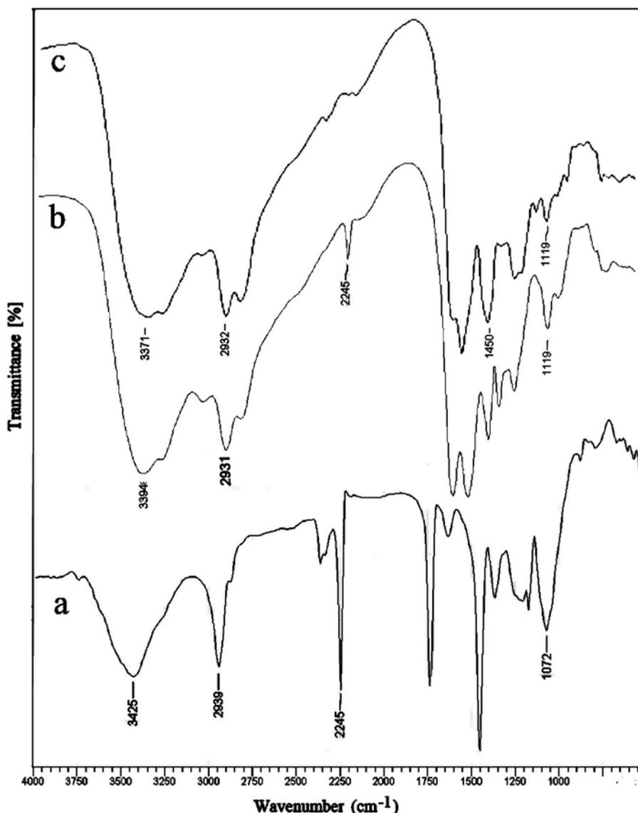
Fig. 1. FT-IR spectra of (a) PAN, (b) PAN-TETA 50, and (c) PAN-TETA 100.
