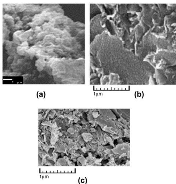
Fig. 8. SEM images of (a) PAN–TETA, (b) PAN–TETA Ag (I), and (c) PAN–TETA Pb(II).
