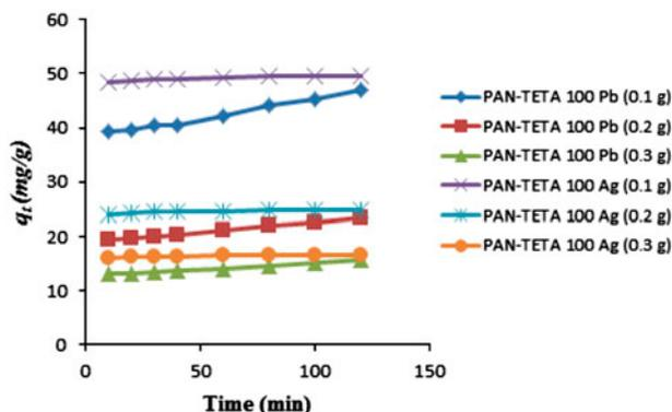
Fig. 3. Effect of adsorbent dose on adsorption of silver and lead ions onto PAN-TETA ( $T=20^{\circ}\text{C}$ ,  $[\text{metal ions}]_0=50\text{ mg L}^{-1}$ ,  $\text{pH}=6$ ).
