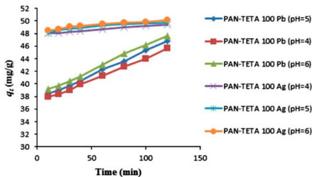
Fig. 2. Effect of contact time and initial pH on the removal rate of silver and lead ions onto PAN-TETA from aqueous solutions ( $T=20^{\circ}\text{C}$ ,  $[\text{metal ion}]_0=50\text{ mg L}^{-1}$ , PAN-TETA = 0.1 g).
