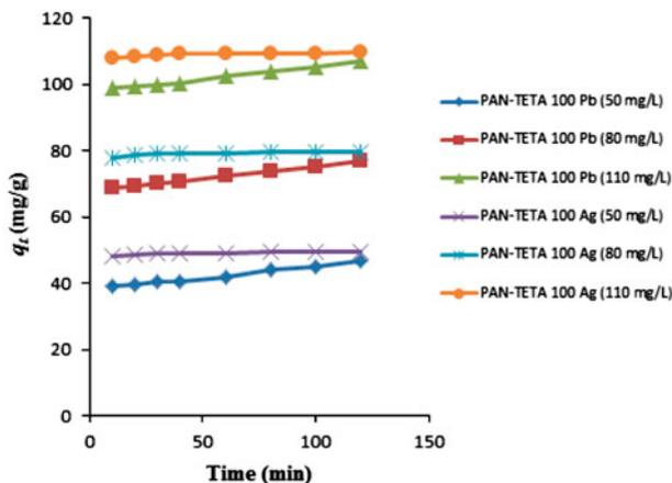
Fig. 4. Effect of contact time and initial concentration of silver and lead ions onto PAN-TETA from aqueous solutions ( $[\text{metal ions}]_0=50, 80$  and  $110\text{ mg L}^{-1}$ ,  $T=20^{\circ}\text{C}$ ,  $\text{pH}=6$ ).
