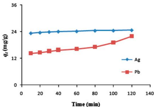
Fig. 12. Effect of contact time on the removal efficiency of silver and lead ions at room temperature ( $[\text{metal ions}]_0 = 50 \text{ mg L}^{-1}$ , PAN-TETA = 0.1 g, pH = 6.0).
