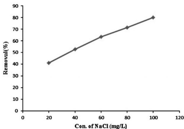
Fig. 6. Effect of ionic strength on the adsorption of lead ion onto PAN–TETA 100 (pH=6, PAN–TETA=0.1 g, agitation time = 1 h,  $T = 20^{\circ}\text{C}$ ,  $[\text{metal ions}]_0 = 25 \text{ mg L}^{-1}$ ).
