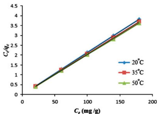
Fig. 11. Langmuir plot of adsorption of lead ions onto PAN-TETA at various temperatures (PH=6, PAN-TETA=0.1 g,  $[\text{metal ions}]_0 = 20, 60, 100, 140, \text{ and } 180 \text{ mg L}^{-1}$ ).
