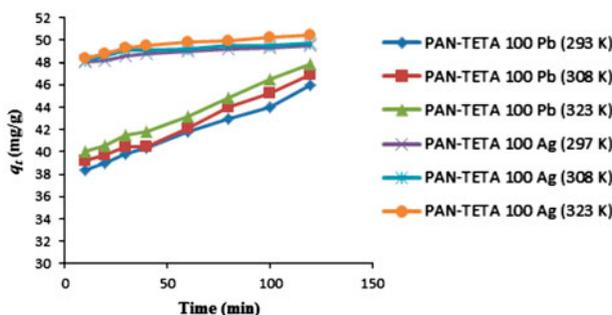
Fig. 5. Effect of contact time and temperature on the removal efficiency of silver and lead ions onto PAN-TETA from aqueous solutions ( $[\text{metal ions}]_0=50\text{ mg L}^{-1}$ ,  $\text{pH}=6$ , PAN-TETA = 0.1 g).
