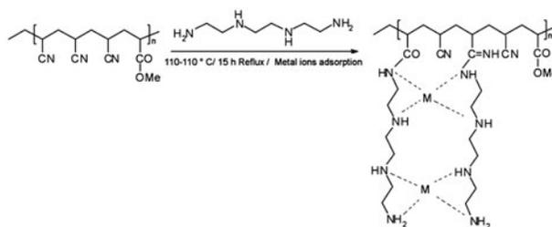
Fig. 7. Scheme of PAN–TETA 50 synthesized and the interaction with metal ions (M).
