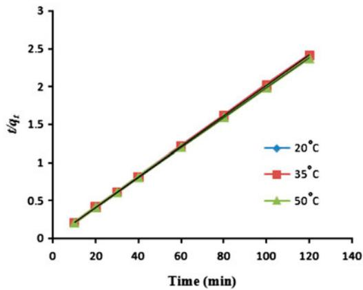
Fig. 9. Pseudo-second-order plots for the adsorption of lead ions onto PAN-TETA at various temperatures ( $[metal\ ions]_0 = 50\ mg\ L^{-1}$ , PAN-TETA = 0.1 g, pH = 6).
