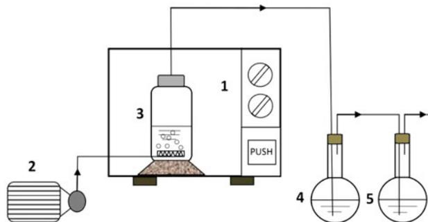
Fig. 1. Schematic diagram of the microwave reactor system. (1) MW oven, (2) air compressor, (3) glass column, (4) and (5) absorption vessel filled with NaOH solution.
