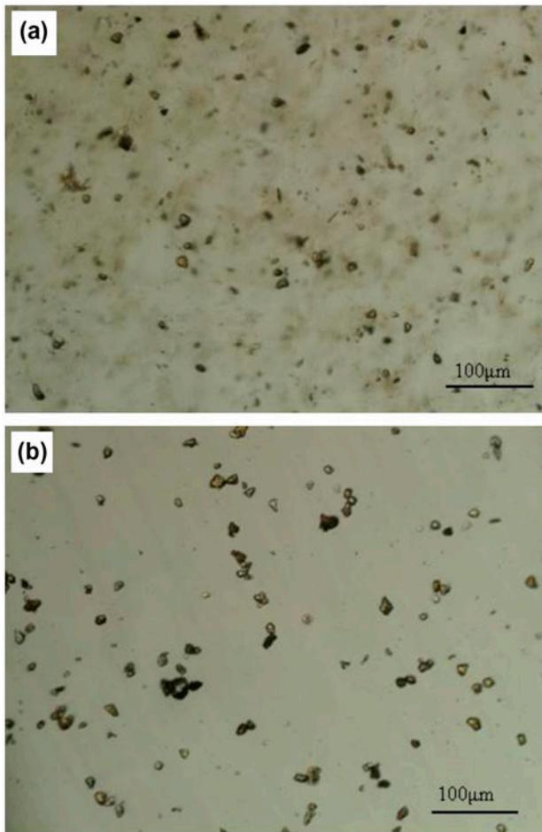
Fig. 4. Images of the flocs: (a) flocculation basin and (b) sedimentation tank.
