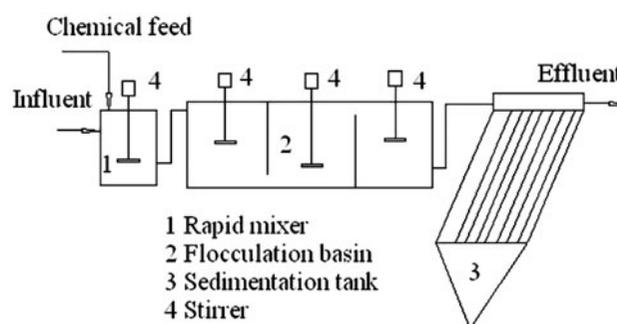
Fig. 1. Experimental apparatus for coagulation.
