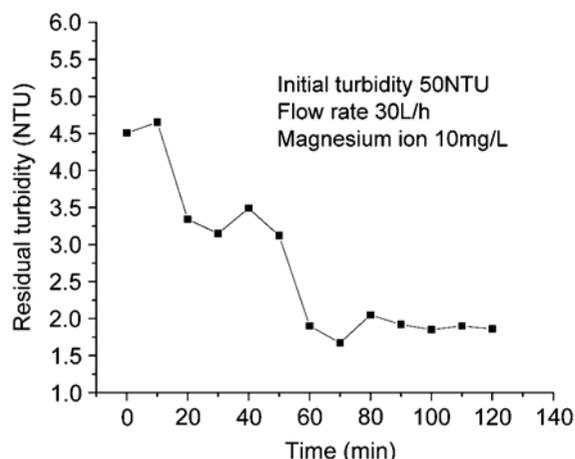
Fig. 2. The residual turbidity changes with time.
