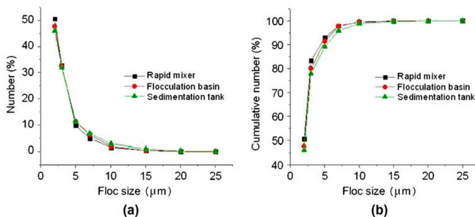
Fig. 3. FSD for three stages: (a) number percentage and (b) cumulative percentage.
