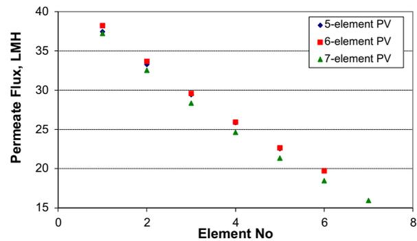
Fig. 6. Profile of mean permeate flux of each SWM element in a pressure vessel, for three cases; i.e. plants with 5-, 6- or 7-element pressure vessels.
