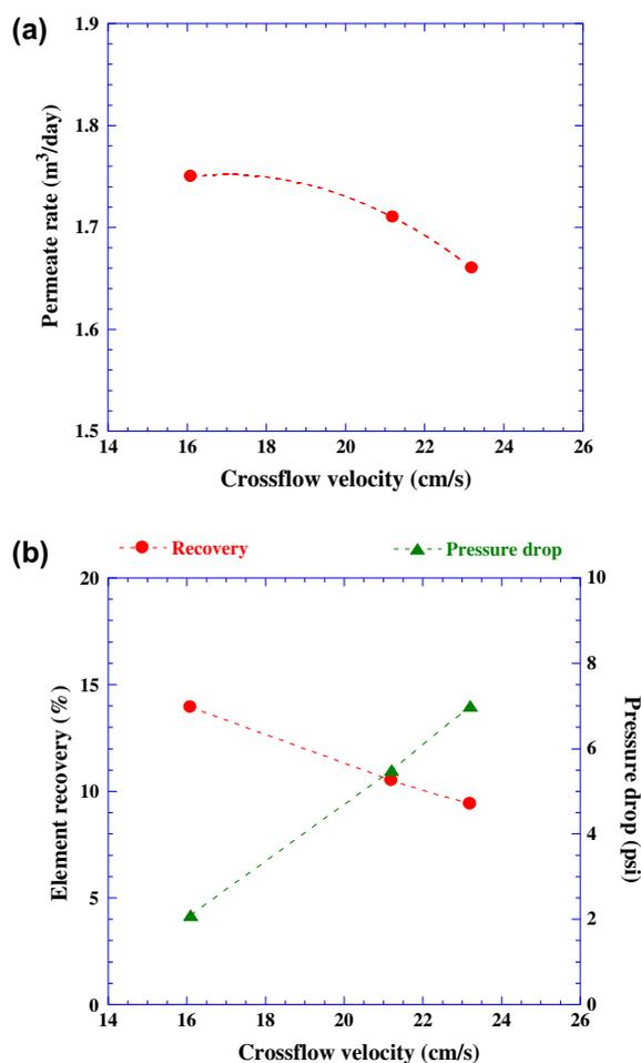
Fig. 3. Experimental data on the effect of cross-flow velocity on membrane performance. Effect on a) SWM element permeate rate and b) SWM element recovery and pressure drop. The plotted cross-flow velocity is an average value of the respective SWM inlet and outlet cross-flow velocities.
