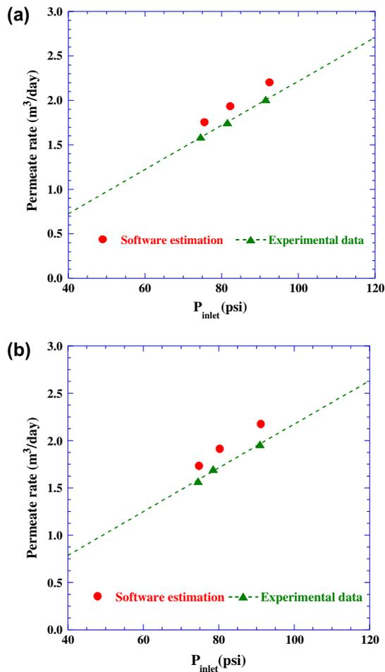
Fig. 4. Comparison of experimental data on performance characteristics with theoretical estimates (obtained with the commercial design software ROSA) for the low-pressure membrane (Filmtec XLE). Average cross-flow velocity: a) 17.5 cm/s and b) 19 cm/s.
