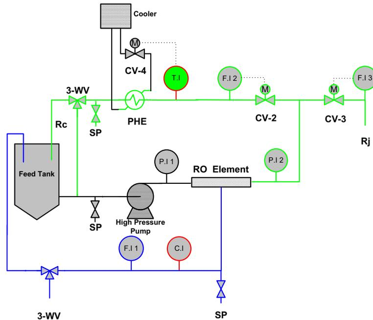
Fig. 2. Schematic diagram of the pilot unit for testing SWM desalination performance.
