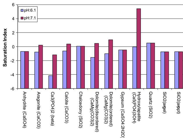
Fig. 5. Saturation indices of solid phases in the retentate stream for untreated and treated (acidified) feedwater; pH values in exiting retentate stream, 7.1 and 6.1 for untreated and treated feed, respectively.
