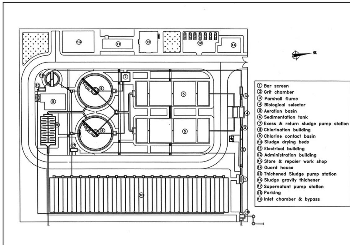
Fig. 3. Wastewater treatment in EAAS plant.
