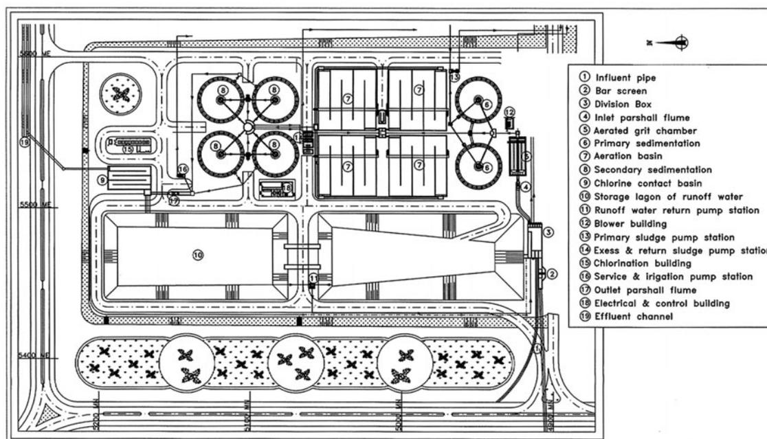
Fig. 2. Wastewater treatment in CAS plant.
