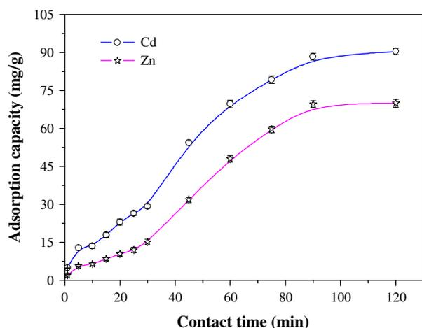
Fig. 4. Adsorption capacity of Zn (II) and Cd (II) onto PS-DETA resin as a function of contact time.
