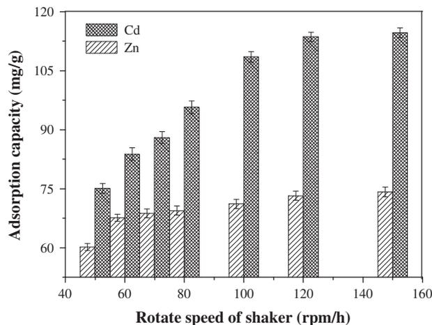
Fig. 3. Adsorption capacity of Zn (II) and Cd (II) onto PS-DETA resin as a function of agitation speed.
