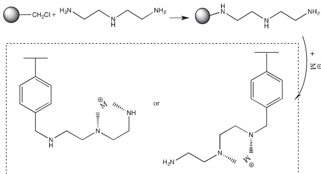
Fig. 1. Synthetic route of PS-DETA resins and possible chelating mechanisms (M: metal ions).
