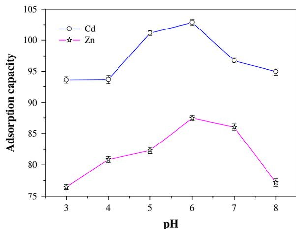
Fig. 2. Adsorption capacity of Zn (II) and Cd (II) onto PS-DETA resin as a function of pH.
