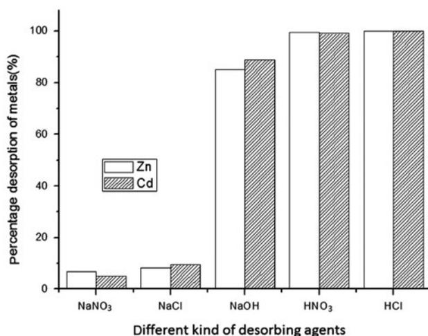
Fig. 9. Desorption of Zn (II) and Cd (II) from PS-DETA resins using various agents.
