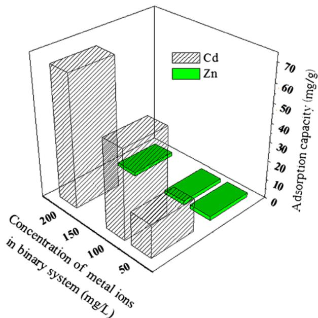
Fig. 6. Competitive adsorption of Zn (II) and Cd (II) onto PS-DETA resin in binary system.
