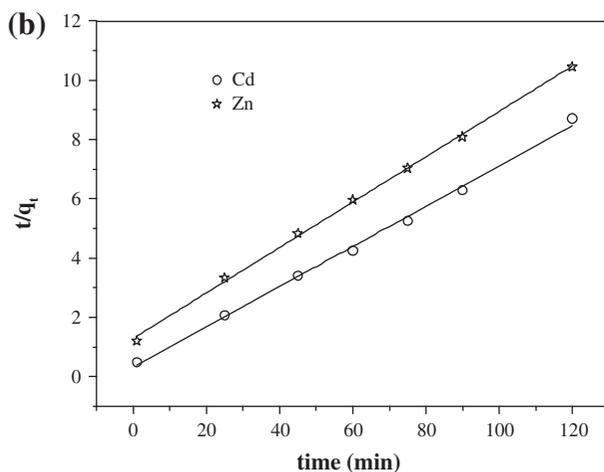
Fig. 8. Adsorption kinetics ((a) pseudo-first order and (b) pseudo-second order) of Zn (II) and Cd (II) onto PS-DETA resin under pH 6.0.
