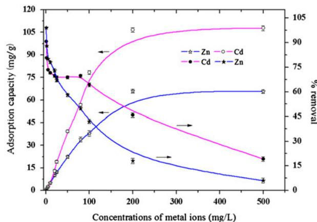
Fig. 5. Adsorption capacity of Zn (II) and Cd (II) onto PS-DETA resin as a function of initial concentration.
