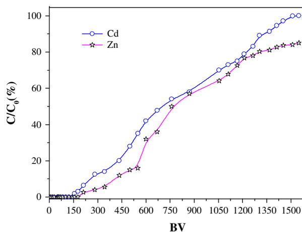
Fig. 10. Breakthrough curves for Zn (II) and Cd (II) removal by PS-DETA resins from industrial wastewater.
