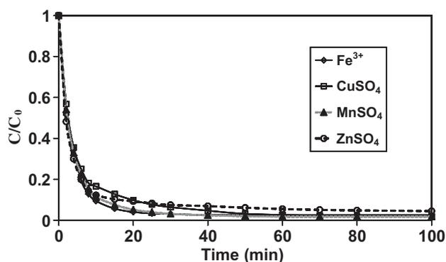
Fig. 8. Effect of Metal on electro-Fenton degradation of NBB.  $C_0=0.05 \text{ mM}$ ,  $[\text{Na}_2\text{SO}_4]=0.5 \text{ M}$ ,  $T=20^\circ\text{C}$ ,  $\text{pH}=2$ ,  $[\text{Fe}^{3+}]=0.05 \text{ mM}$ ,  $I=150 \text{ mA}$ .
