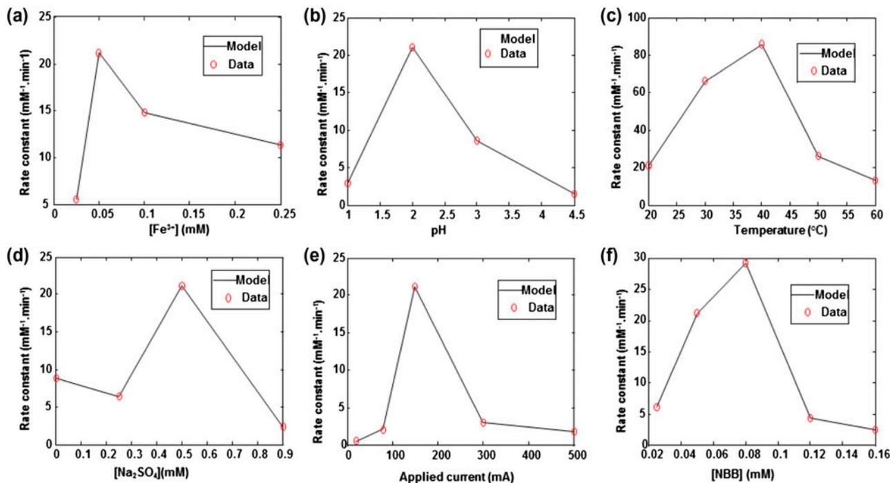
Fig. 5. Simulation and experimental data of the evolution of rate constant. (Initial conditions:  $C_0=0.05$  mM,  $[\text{Na}_2\text{SO}_4]=0.5$  M,  $T=20^\circ\text{C}$ ,  $\text{pH}=2$ ,  $I=150$  mA.)
