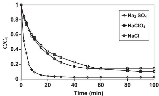
Fig. 7. Effect of supporting electrolyte species on electro-Fenton degradation of NBB.  $C_0=0.05$  mM,  $[\text{Na}_2\text{SO}_4]=0.5$  M,  $T=20^\circ\text{C}$ ,  $\text{pH}=2$ ,  $[\text{Fe}^{3+}]=0.05$  mM,  $I=150$  mA.
