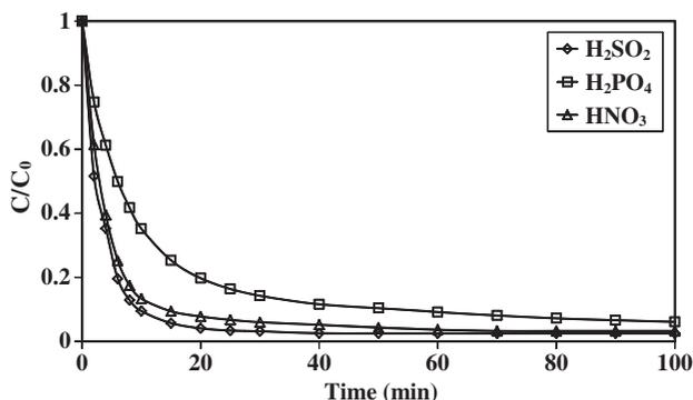
Fig. 6. Effect of the nature of the acid used to adjust the pH on electro-Fenton degradation of NBB  $C_0=0.05$  mM,  $[\text{Na}_2\text{SO}_4]=0.5$  M,  $T=20^\circ\text{C}$ ,  $\text{pH}=2$ ,  $[\text{Fe}^{3+}]=0.05$  mM,  $I=150$  mA.
