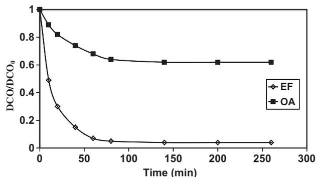
Fig. 11. Mineralization of NBB by various oxidation processes.  $C_0=0.05$  mM,  $[\text{Na}_2\text{SO}_4]=0.5$  M,  $T=20^\circ\text{C}$ ,  $\text{pH}=2$ ,  $[\text{Fe}^{3+}]=0.05$  mM,  $I=150$  mA.
