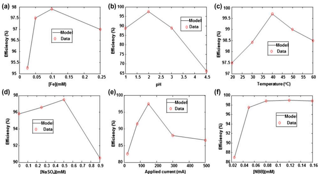
Fig. 4. Simulation and experimental data of the evolution of degradation efficiency. (Initial conditions:  $C_0 = 0.05$  mM,  $[\text{Na}_2\text{SO}_4] = 0.5$  M,  $T = 20^\circ\text{C}$ ,  $\text{pH} = 2$ ,  $I = 150$  mA.)
