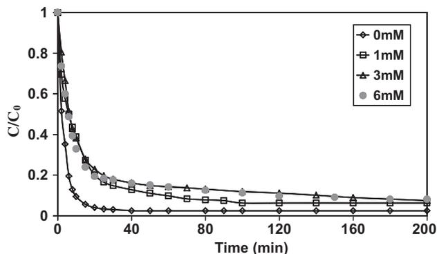
Fig. 10. Effect of tert-butyl alcohol on electro-Fenton degradation of NBB.  $C_0=0.05$  mM,  $[\text{Na}_2\text{SO}_4]=0.5$  M,  $T=20^\circ\text{C}$ ,  $\text{pH}=2$ ,  $[\text{Fe}^{3+}]=0.05$  mM,  $I=150$  mA.
