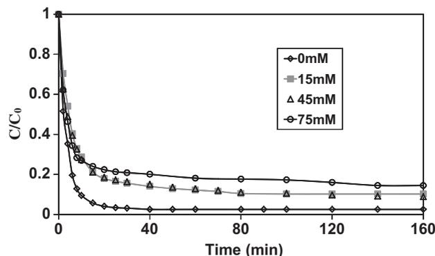
Fig. 9. Effect of sucrose addition on electro-Fenton degradation of NBB.  $C_0=0.05 \text{ mM}$ ,  $[\text{Na}_2\text{SO}_4]=0.5 \text{ M}$ ,  $T=20^\circ\text{C}$ ,  $\text{pH}=2$ ,  $[\text{Fe}^{3+}]=0.05 \text{ mM}$ ,  $I=150 \text{ mA}$ .
