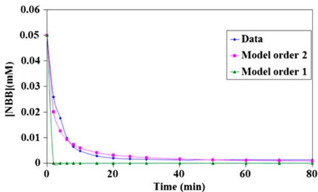
Fig. 2. Degradation kinetic of NBB by electro-Fenton process, the comparison of model and experimental data for second order.
