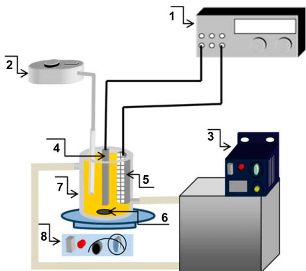
Fig. 1. The schematic view of the undivided lab electrolysis cell system: (1) supply source, (2) air pump, (3) thermostatic bath, (4) carbon-felt cathode, (5) platinum anode, (6) magnet, (7) electrolysis cell, and (8) magnetic stirrer.
