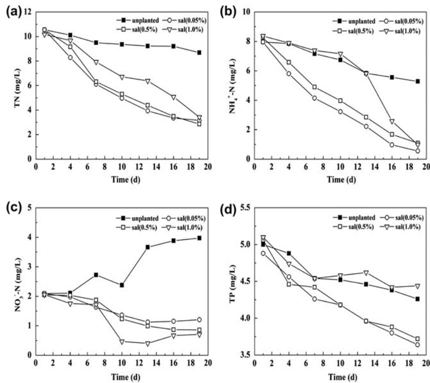
Fig. 1. The profile of TN(a),  $\text{NH}_4^+\text{-N}$ (b),  $\text{NO}_3^-\text{-N}$ (c), and TP(d) in planted *L. salicaria* microcosm systems for the treatment of eutrophic water with different salinities during the experiment.
