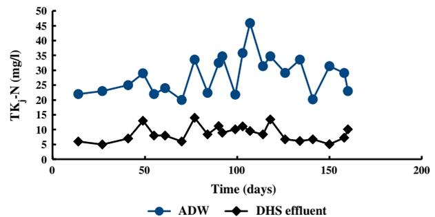
Fig. 4. Time course of  $TKj-N$  in the influent and the effluent of DHS system treating ADW at OLR of  $3.0 \text{ kg COD/m}^3 \text{ d}$ .
