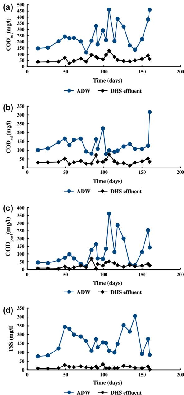
Fig. 2(a)–(d). Variation of  $COD_{tot}$ ,  $COD_{sol}$ ,  $COD_{part}$ , and TSS in the influent and the effluent of DHS system treating ADW.
