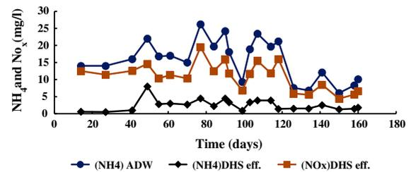
Fig. 3. Nitrification efficiency of the DHS system treating ADW at OLR of  $3.0 \text{ kg COD/m}^3 \text{ d}$ .
