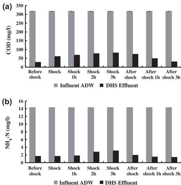
Fig. 6(a) and (b). Effect of the hydraulic shock load on the COD and ammonia–nitrogen removal in the DHS system treating ADW.
