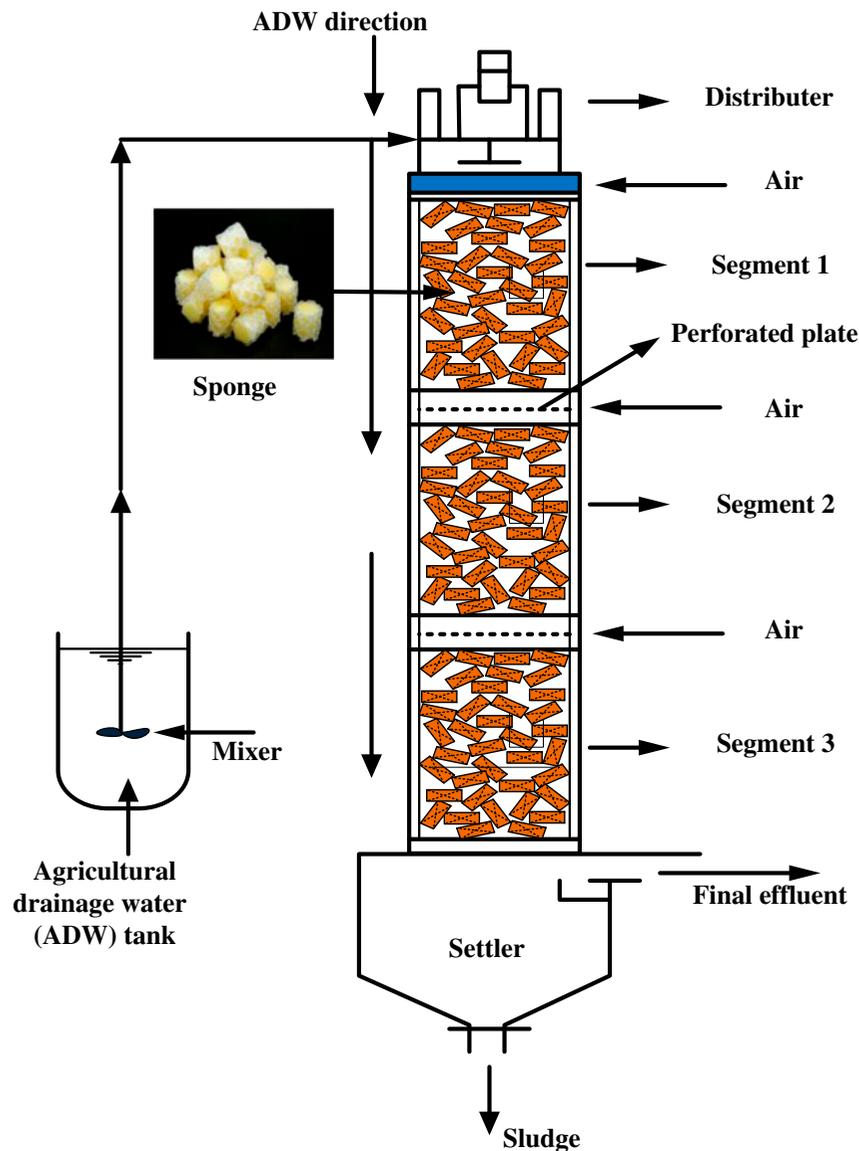
Fig. 1. Schematic diagram for the experimental setup of the DHS system fed with ADW.
