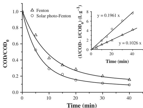
Fig. 10. Trend of COD/COD<sub>0</sub> ratio during the oxidation of chlorpyrifos solution by Fenton and solar photo-Fenton reactions. The inset panel shows the fitting of the experimental data to a second-order reaction kinetic model for the two processes. H<sub>2</sub>O<sub>2</sub> dosing rate = 50 mg min<sup>-1</sup>; [Fe<sup>2+</sup>]<sub>0</sub> = 2.0 mM; COD<sub>0</sub> = 1,300 mg L<sup>-1</sup>; pH = 3.0; and T = 40 °C.
