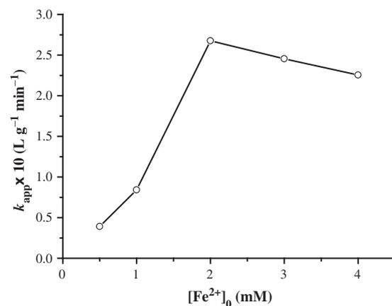
Fig. 5. *k<sub>app</sub>* evolution at different initial Fe<sup>2+</sup> concentration. COD<sub>0</sub>=930 mg L<sup>-1</sup>; H<sub>2</sub>O<sub>2</sub> dosing rate=40 mg min<sup>-1</sup>; pH=3.0; and *T*=25 °C.
