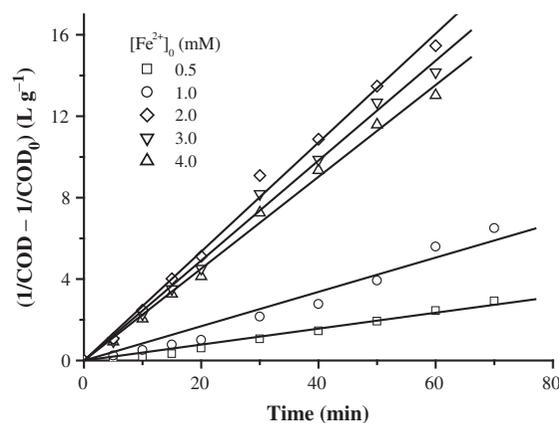
Fig. 4. Plot of  $(1/\text{COD} - 1/\text{COD}_0) - t$  at different initial Fe<sup>2+</sup> concentration. COD<sub>0</sub>=930 mg L<sup>-1</sup>; H<sub>2</sub>O<sub>2</sub> dosing rate=40 mg min<sup>-1</sup>; pH=3.0; and *T*=25 °C.
