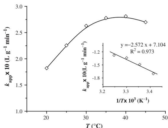
Fig. 9. Evolution of  $k_{app}$  at different temperatures. The inset shows the plot of  $\ln k_{app} - (1/T)$ .  $COD_0 = 930 \text{ mg L}^{-1}$ ;  $H_2O_2$  dosing rate =  $40 \text{ mg min}^{-1}$ ;  $[Fe^{2+}]_0 = 2.0 \text{ mM}$ ; and pH = 3.0.
