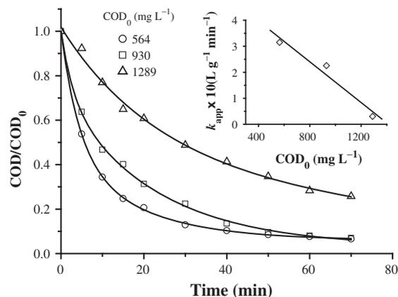
Fig. 7. Effect of initial chlorpyrifos concentration on the COD removal by the Fenton process. The inset panel shows  $k_{\text{app}}$  evolution at different initial COD.  $\text{H}_2\text{O}_2$  dosing rate =  $40 \text{ mg min}^{-1}$ ;  $[\text{Fe}^{2+}]_0 = 2.0 \text{ mM}$ ;  $\text{pH} = 3.0$ ; and  $T = 25^\circ\text{C}$ .
