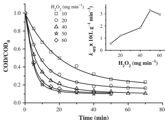
Fig. 6. Effect of  $\text{H}_2\text{O}_2$  dosing rate on the trend of  $\text{COD}/\text{COD}_0$  ratio during the oxidation of chlorpyrifos solution by Fenton process.  $[\text{Fe}^{2+}]_0 = 2.0 \text{ mM}$ ;  $\text{COD}_0 = 930 \text{ mg L}^{-1}$ ,  $\text{pH} = 3.0$ ; and  $T = 25^\circ\text{C}$ .
