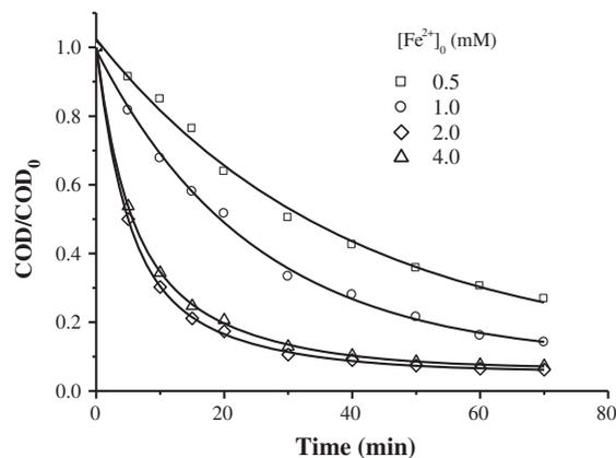
Fig. 3. Effect of initial  $\text{Fe}^{2+}$  concentration on the COD removal by Fenton process. The inset panel shows  $k_{\text{app}}$  evolution at different  $\text{Fe}^{2+}$  concentrations.  $\text{COD}_0 = 930 \text{ mg L}^{-1}$ ;  $\text{H}_2\text{O}_2$  dosing rate =  $40 \text{ mg min}^{-1}$ ; pH = 3.0; and  $T = 25^\circ\text{C}$ .
