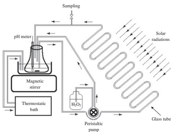
Fig. 2. Scheme of the experimental installation.
