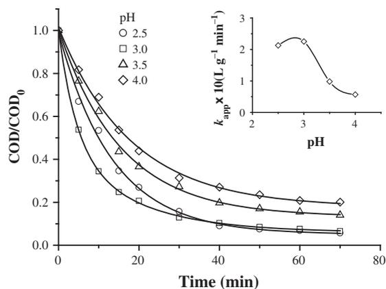
Fig. 8. Effect of initial pH on the COD removal by the Fenton process. The inset panel shows  $k_{app}$  evolution at different pH.  $H_2O_2$  dosing rate =  $40 \text{ mg min}^{-1}$ ;  $[Fe^{2+}]_0 = 2.0 \text{ mM}$ ;  $COD_0 = 930 \text{ mg L}^{-1}$ ; and  $T = 25^\circ\text{C}$ .
