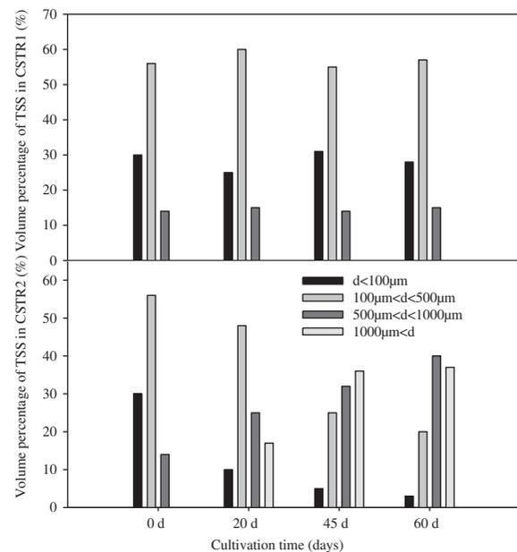
Fig. 2. Evolution of particle size distribution of anaerobic sludge. (Flocculent sludge was the major component in both of the two CSTRs at the beginning of the experiment. After approximately 45 days' cultivation, the sludge in the CSTR2 was almost granulated).
