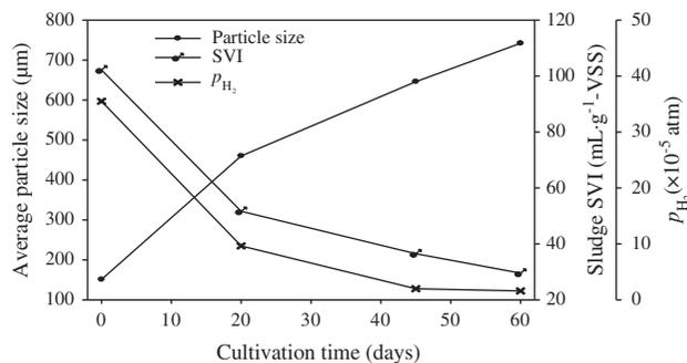
Fig. 5. The relationships between the sludge SVI,  $p_{\text{H}_2}$  and the average particle size in CSTR2.
