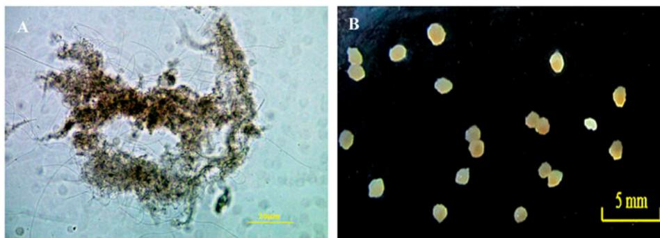
Fig. 6. The sludge morphology after 45 days cultivation: (A) CSTR1, flocculent sludge; (B) CSTR2, granular sludge. (After approximately 45 days cultivation, the sludge formed in these two CSTRs was different significantly. The granular sludge formed in CSTR2 possessed a relatively regular shape and clear outline).
