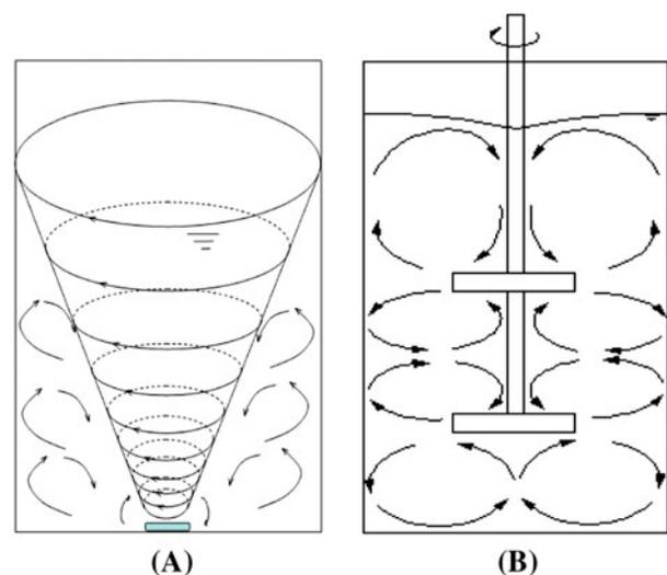
Fig. 1. Streamline maps in: (A) CSTR1; (B) CSTR2. (Compared with magnetic stirring (A), axial-flow mixing (B) could produce good convective mass transfer and it is good at the main circulation).
