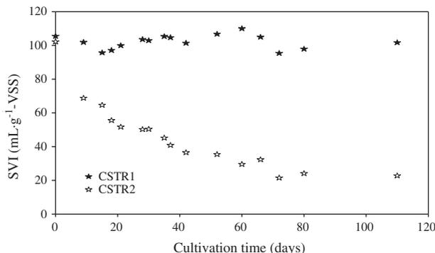
Fig. 3. Changes of sludge settleability (SVI) in the two CSTRs. (Sludge settleability was significantly improved with the sludge granulation of the CSTR2. The sludge SVI in CSTR1 was approximately remained in  $105.5 \text{ mL g}^{-1}$  and the sludge SVI in CSTR2 was decreased from  $102.2$  to  $22.78 \text{ mL g}^{-1}$ ).
