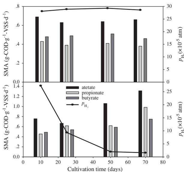
Fig. 4. Changes of  $p_{\text{H}_2}$  and the bacterial activities of the anaerobic sludge in: (A) CSTR1; (B) CSTR2.
