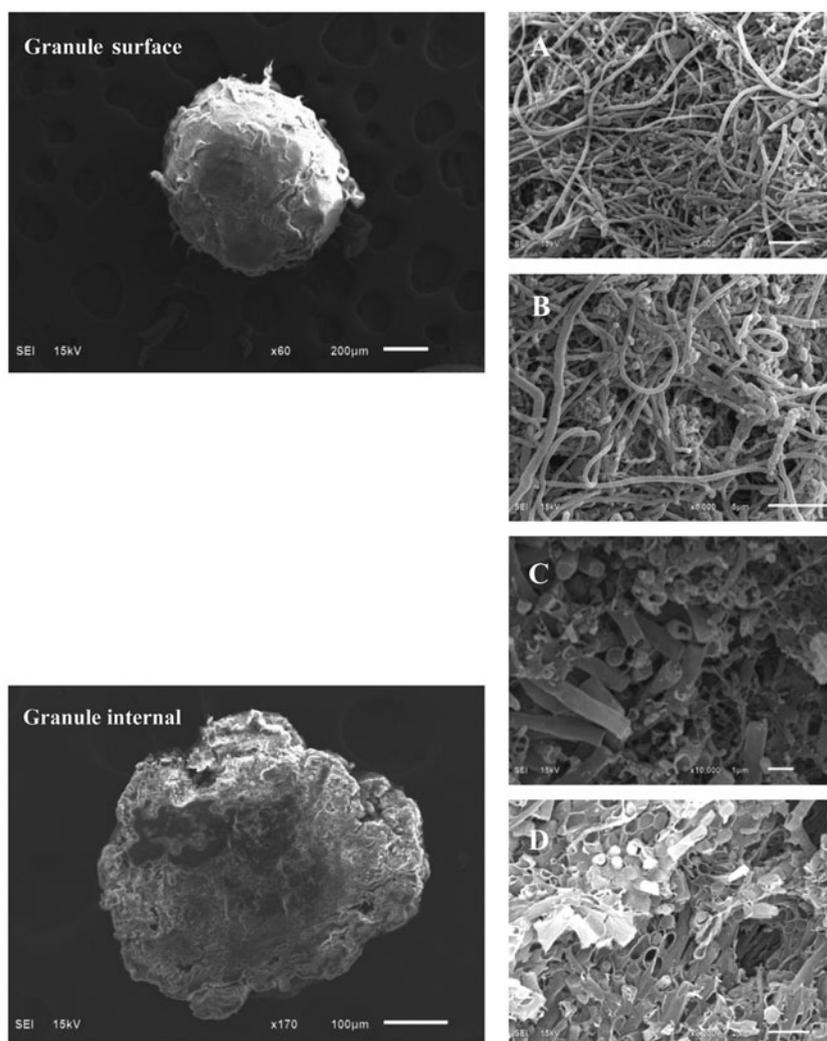
Fig. 7. SEM image of the granular sludge from CSTR2. ((A) and (B): aggregates of filamentous bacterial cells on the surface of the granular sludge; (C) and (D): arrangement of bacterial cells inner the cross-section of the granule surrounded by extracellular polymeric substances (EPS)).
