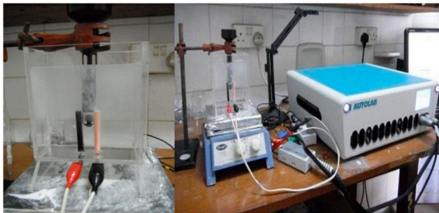
Fig. 7. Developed reactor cell. Volume of the reactor cell = 500 ml. Area of anode and cathode = 10.37 cm 2 .
