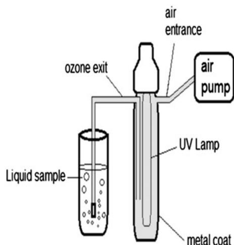
Fig. 2. Schematic of diagram the ozone process.
