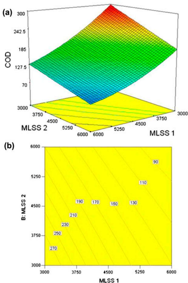
Fig. 6. Response surface and contour plots of COD removal rate without ozonation. Interactive effects of MLSS1 and MLSS2 on COD removal rate ((a) and (b)).
