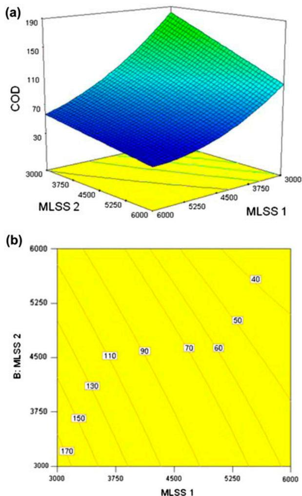
Fig. 7. Response surface and contour plots of COD removal rate with ozonation. Interactive effects of MLSS1 and MLSS2 on COD removal rate ((a) and (b)).
