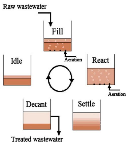
Fig. 1. Schematic diagram of the SBR process.
