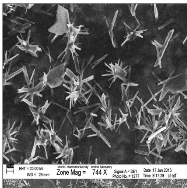
Fig. 9. SEM image of calcium sulfate precipitates [12].
