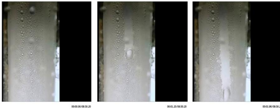
Fig. 6. Drop condensation on the inner surface of the tube.
